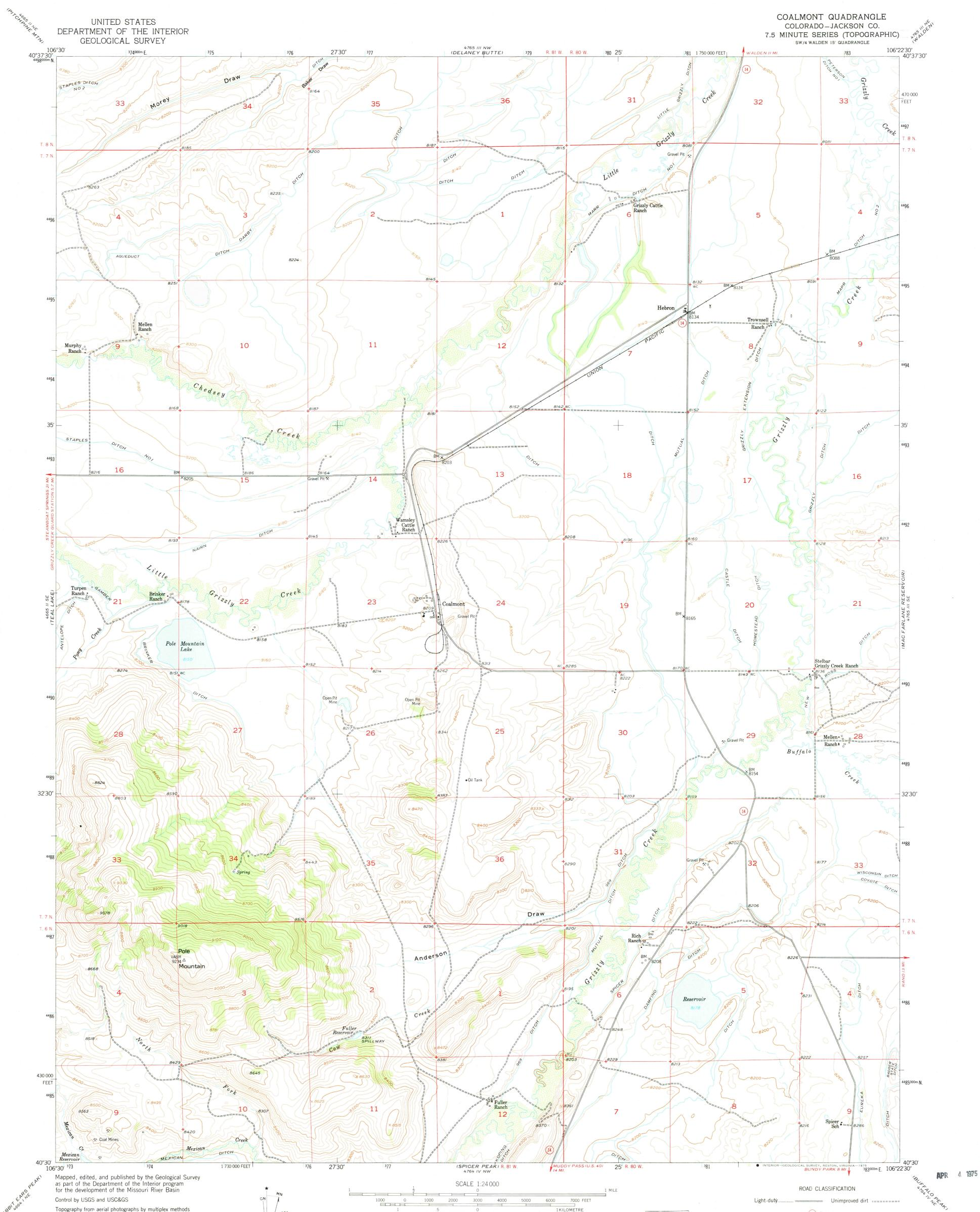
Topography from aerial photograph Aerial photographs taken 1951. Field check 1955 Polyconic projection. 1927 North American datum 10,000 foot grid based on Colorado coordinate system. north zone UTM GRID AND 1955 MAGNETIC NORTH DECLINATION AT CENTER OF SHEET Unchecked elevations are shown in brown 1000-metre Universal Transverse Mercator grid ticks, zone 13, shown in blue
