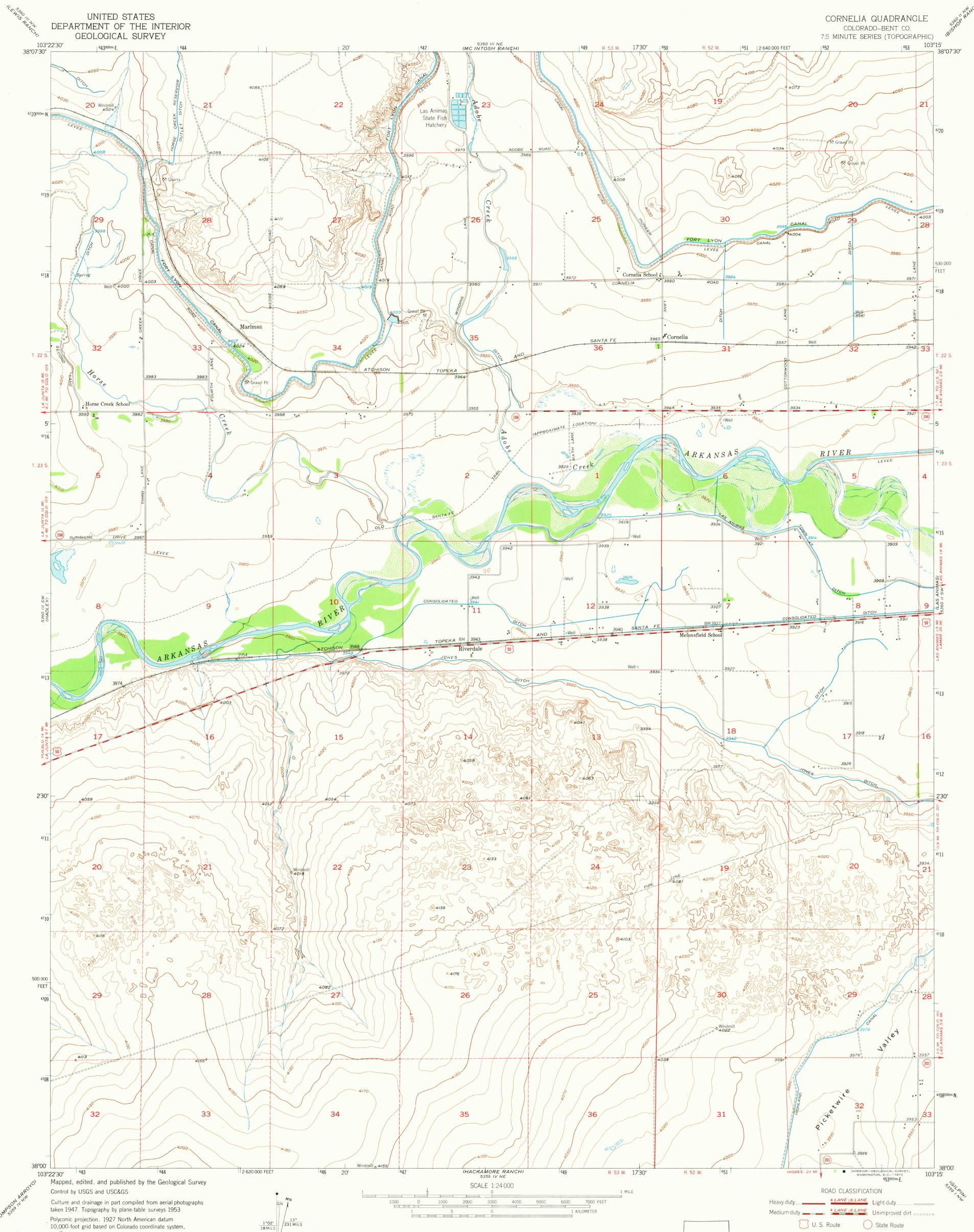
10,000-foot grid based on Colorado coordinate system, south zone
