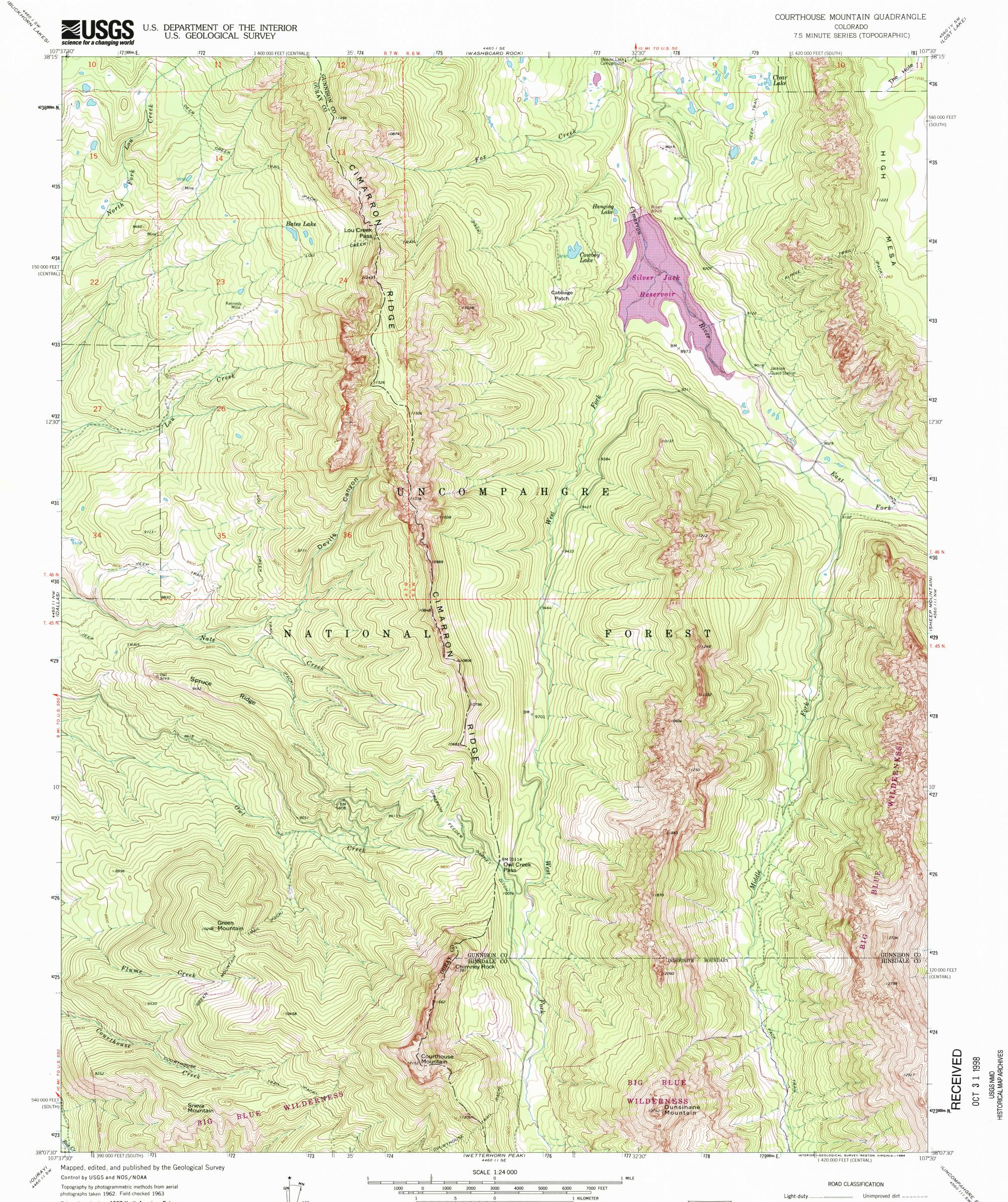
Polyconic projection. 1927 North American Datum 10,000-foot grids based on Colorado coordinate system, south and central zones 1000-meter Universal Transverse Mercator grid ticks, zone 13, shown in blue Where omitted, land lines have not been established or are not shown because of insufficient data To place on the predicted North American Datum 1983
