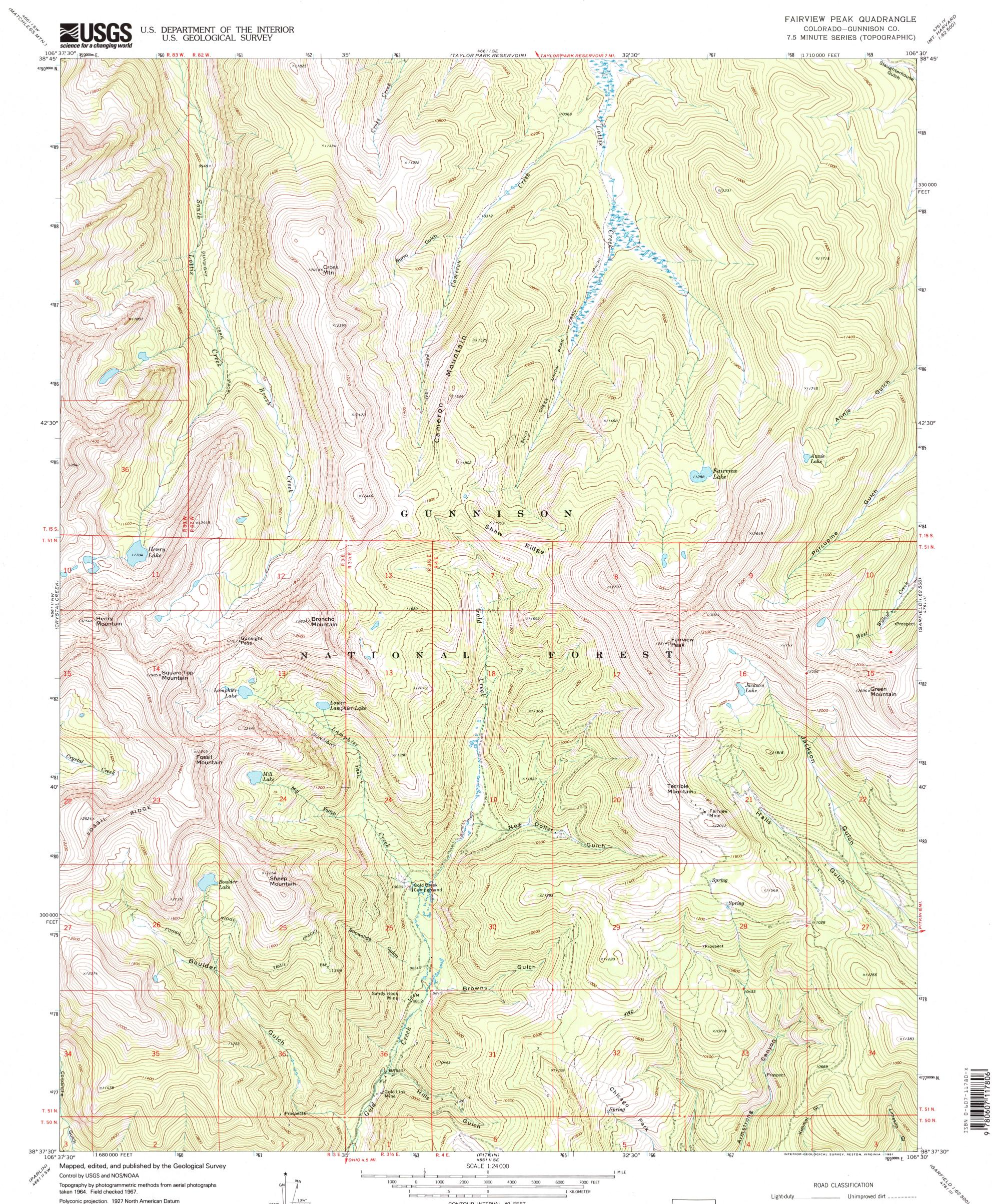
Polyconic projection. 1927 North American Datum 10,000-foot grid based on Colorado coordinate system, central zone 1000-meter Universal Transverse Mercator grid ticks, zone 13, shown in blue The difference between 1927 North American Datum and North American Datum of 1983 (NAD 83) for 7.5 minute intersections is given in USGS Bulletin 1875. The NAD 83 is shown by dashed
