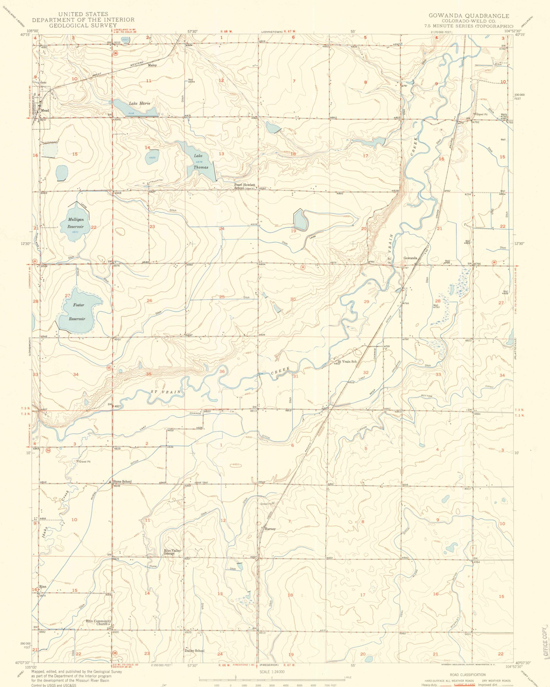
Control by USGS and USC&GS Culture and drainage in part compiled from aerial photographs taken November 1948 Topography by plane-table methods 1949 Polyconic projection. 1927 North American datum 10,000-foot grid based on Colorado coordinate system, north zone
