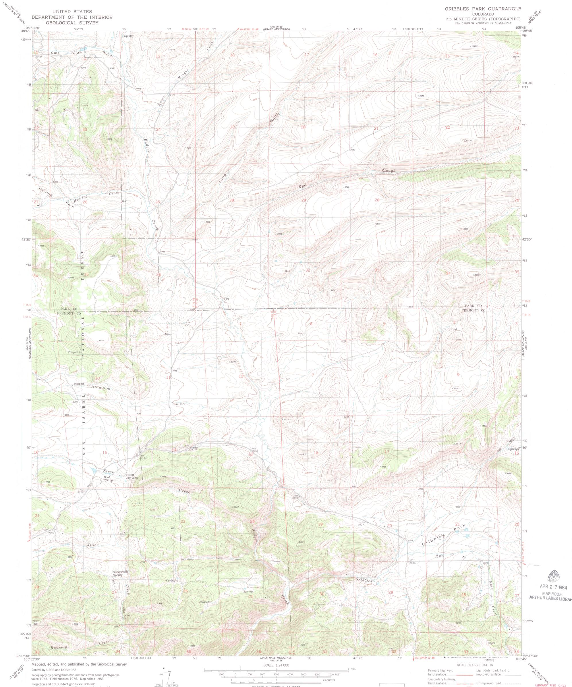
coordinate system, central zone (Lambert conformal conic) 1000-meter Universal Transverse Mercator grid, zone 13 1927 North American datum To place on the predicted North American Datum 1983 move the projection lines 4 meters north and 50 meters east as shown by dashed corner ticks
