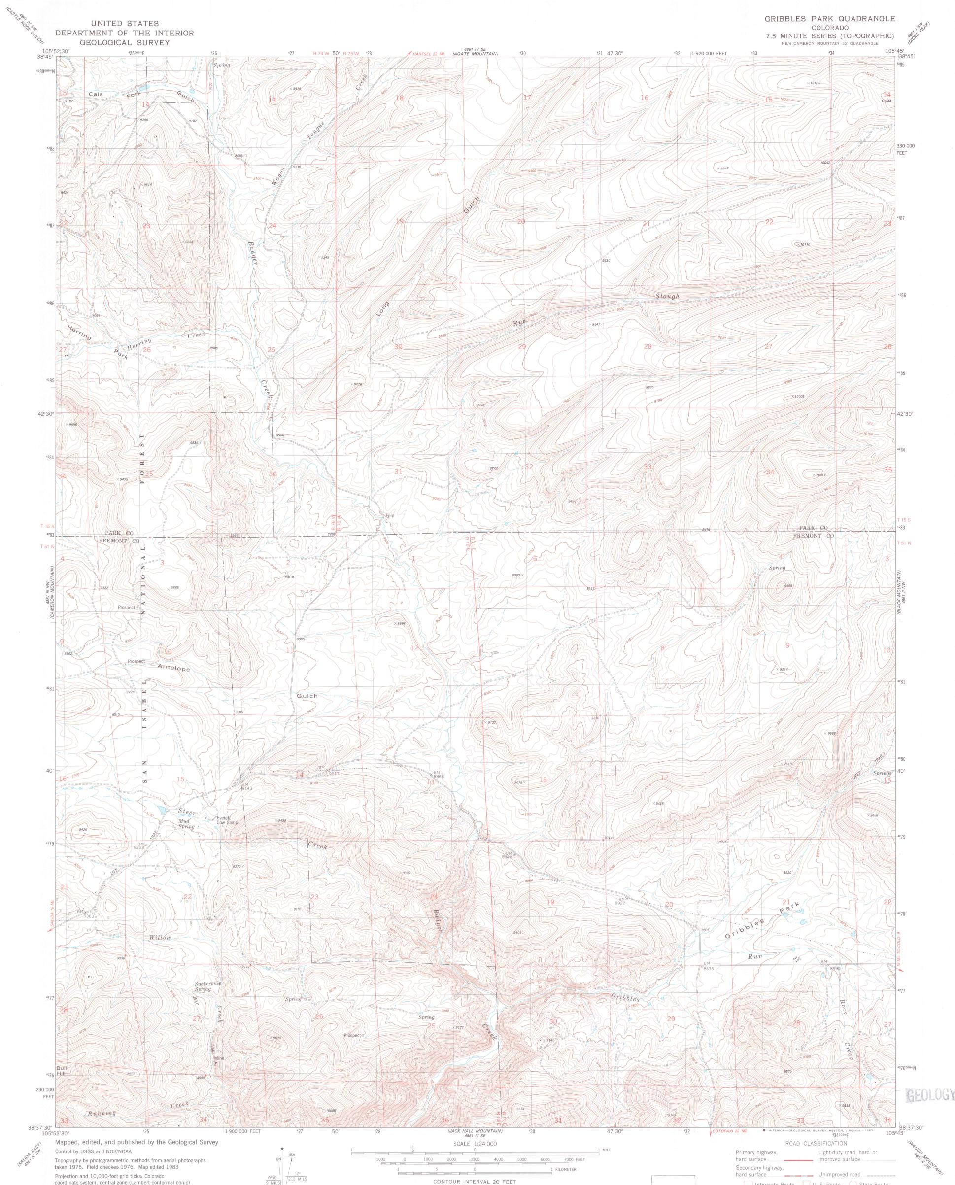
1000-meter Universal Transverse Mercator grid, zone 13 1927 North American datum To place on the predicted North American Datum 1983 move the projection lines 4 meters north and 50 meters east as shown by dashed corner ticks
