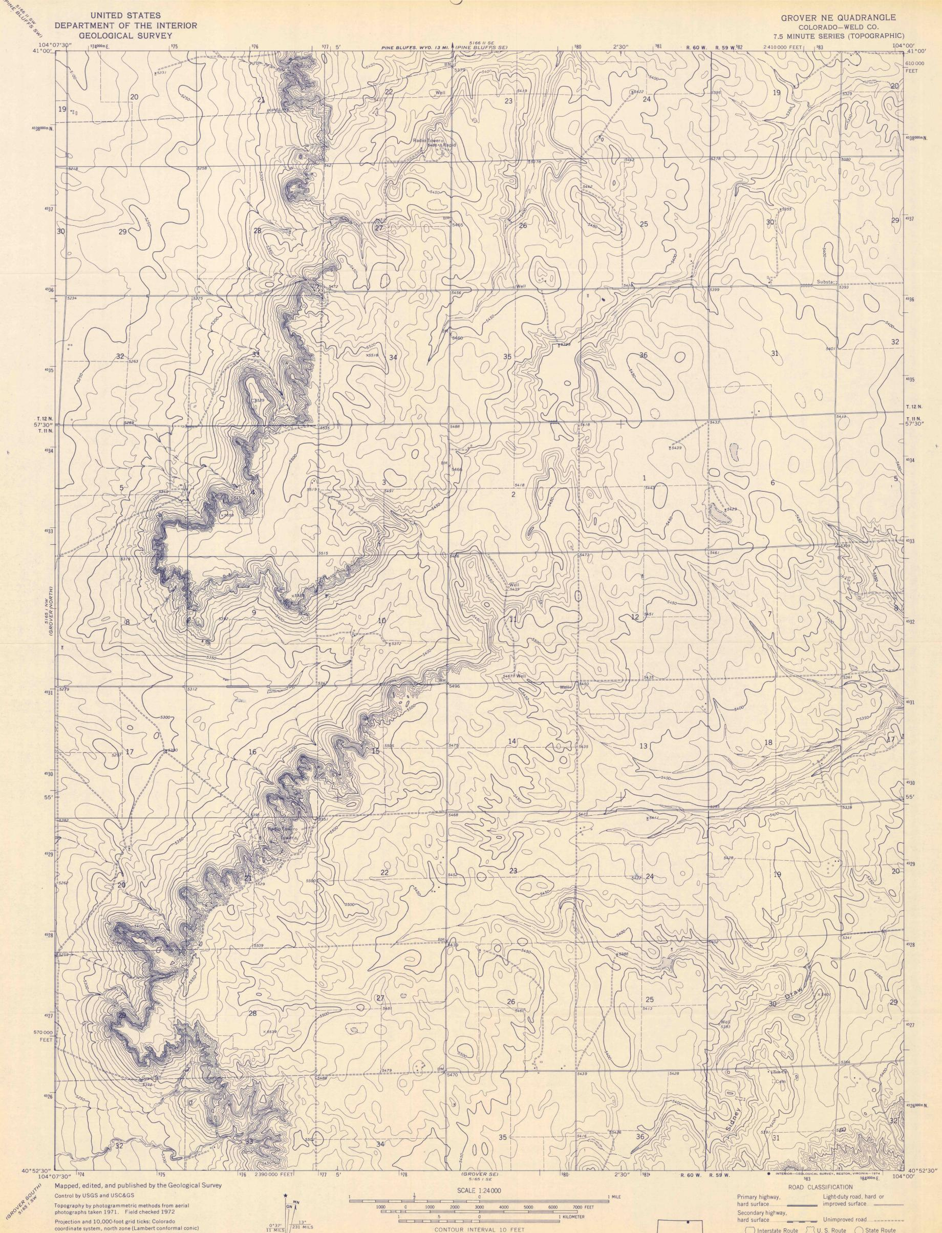
1000-meter Universal Transverse Mercator grid ticks, zone 13, shown in blue. 1927 North American datum Fine red dashed lines indicate selected fence lines Landlines, inpart, are based on cultural development and are not reflected in the original land survey
