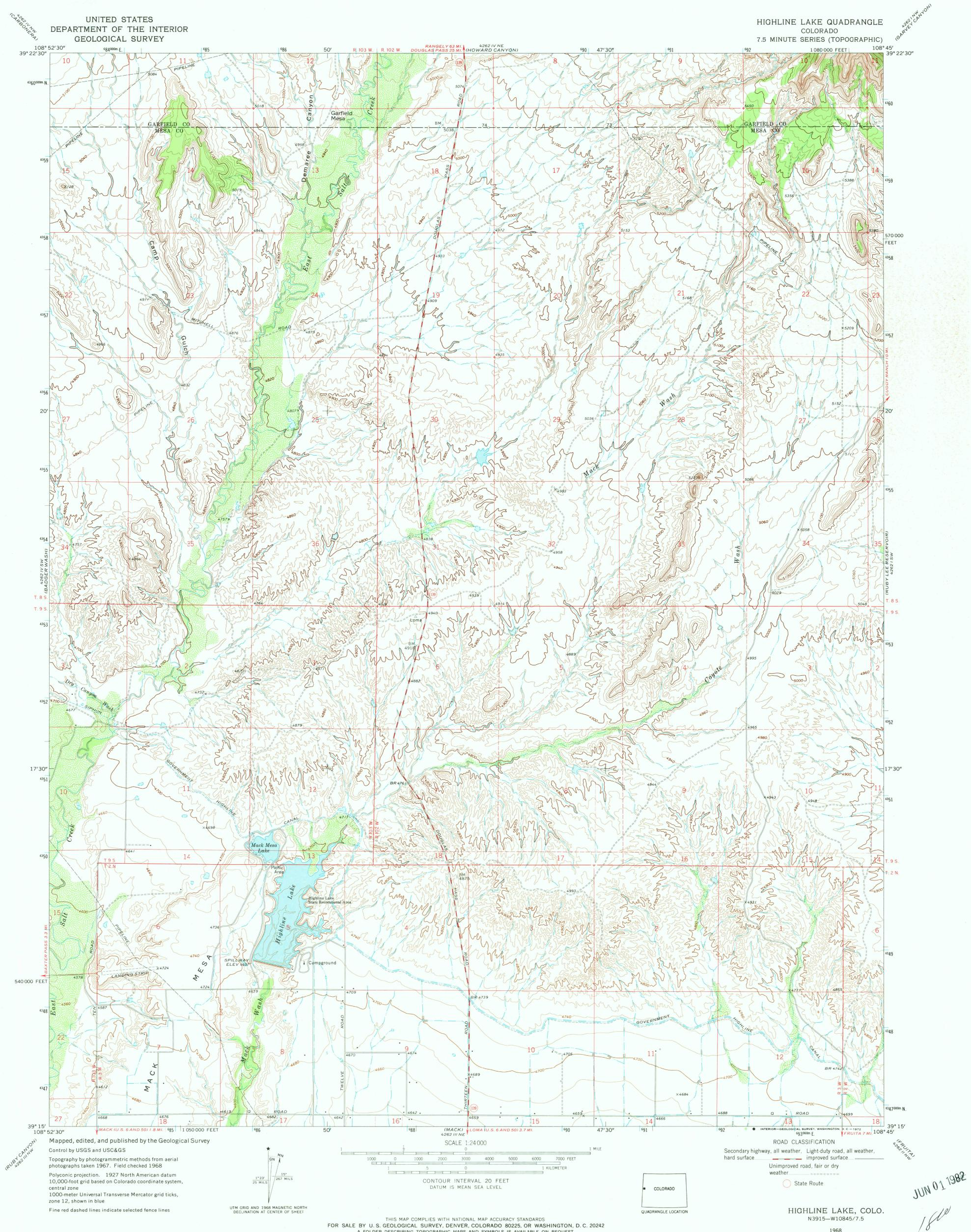
Polyconic projection. 1927 North American datum 10,000-foot grid based on Colorado coordinate system, central zone 1000-meter Universal Transverse Mercator grid ticks, zone 12, shown in blue
