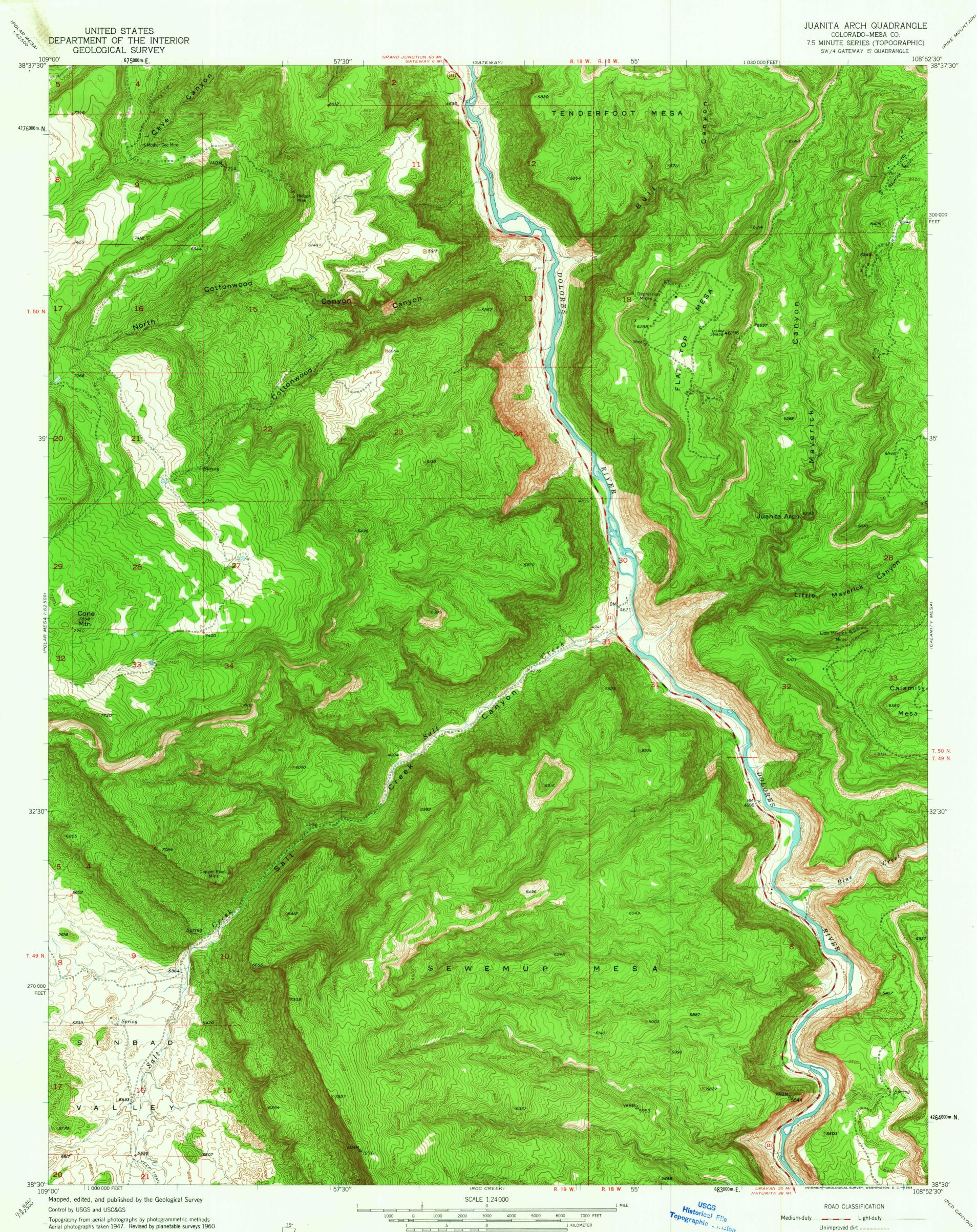
Polyconic projection. 1927 North American datum 10,000-foot grid based on Colorado coordinate system, central zone 1000-meter Universal Transverse Mercator grid ticks, zone 12, shown in blue Dashed land lines indicate approximate locations Land lines unsurveyed in part of T. 49 N.-Rs. 18 and 19 W. and T. 50 N.-Rs. 18 and 19 W.
