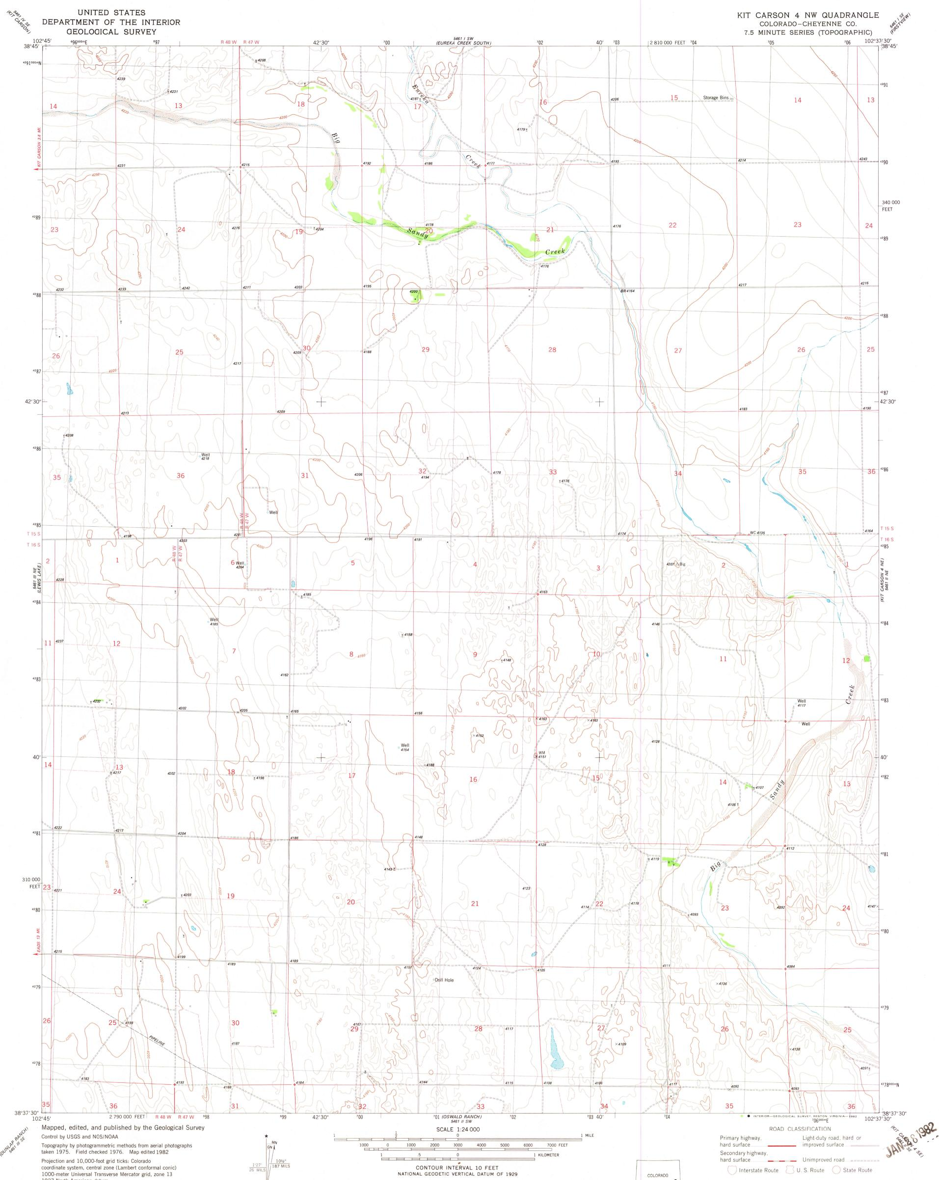
1000-meter Universal Transverse Mercator grid, zone 13 1927 North American datum To place on the predicted North American Datum 1983 move the projection lines 3 meters north and 42 meters east as shown by dashed corner ticks
