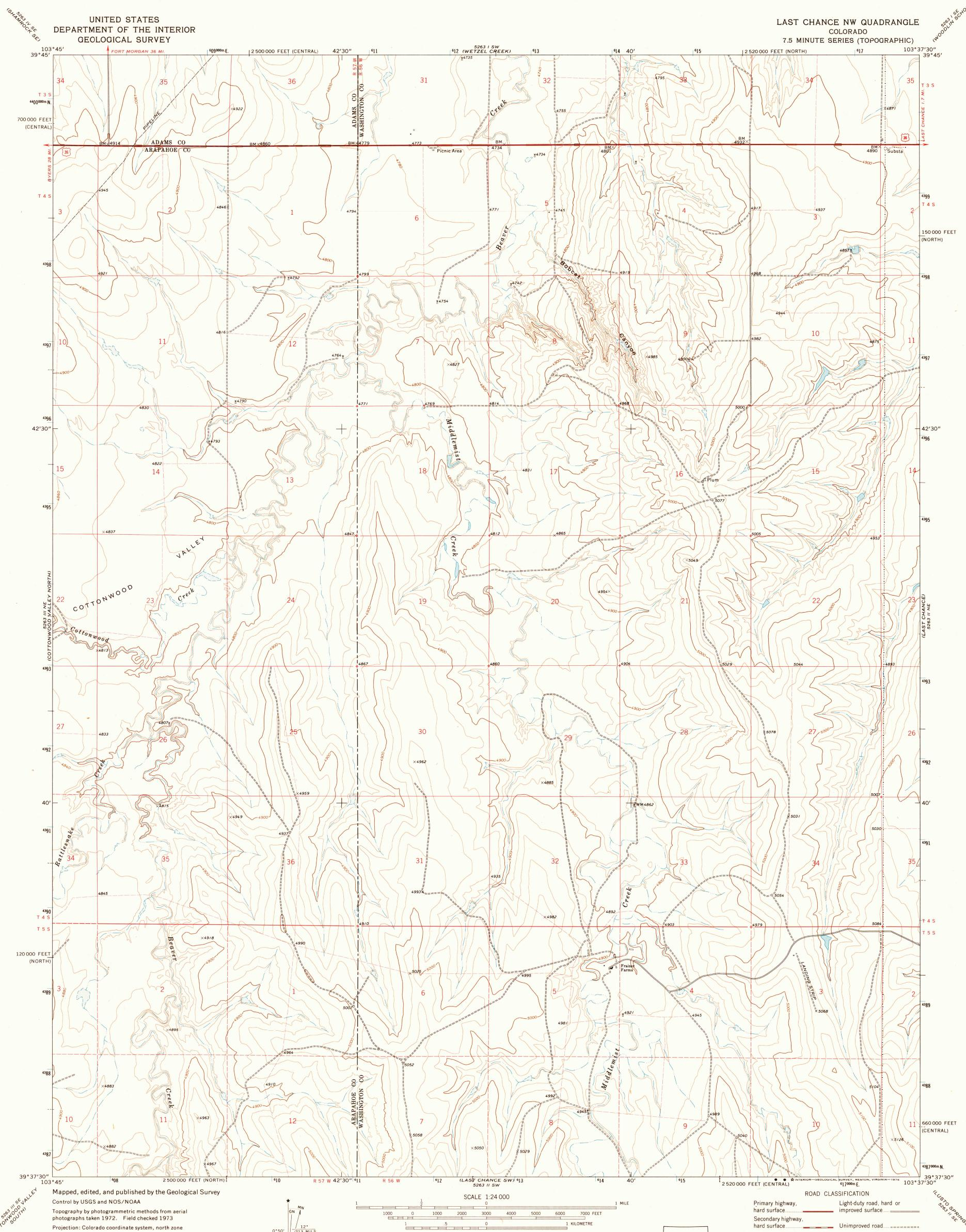
(Lambert conformal conic) 10,000-foot grid ticks based on Colorado coordinate system, north and central zones 1000-metre Universal Transverse Mercator grid ticks, zone 13, shown in blue. 1927 North American datum Fine red dashed lines indicate selected fence lines
