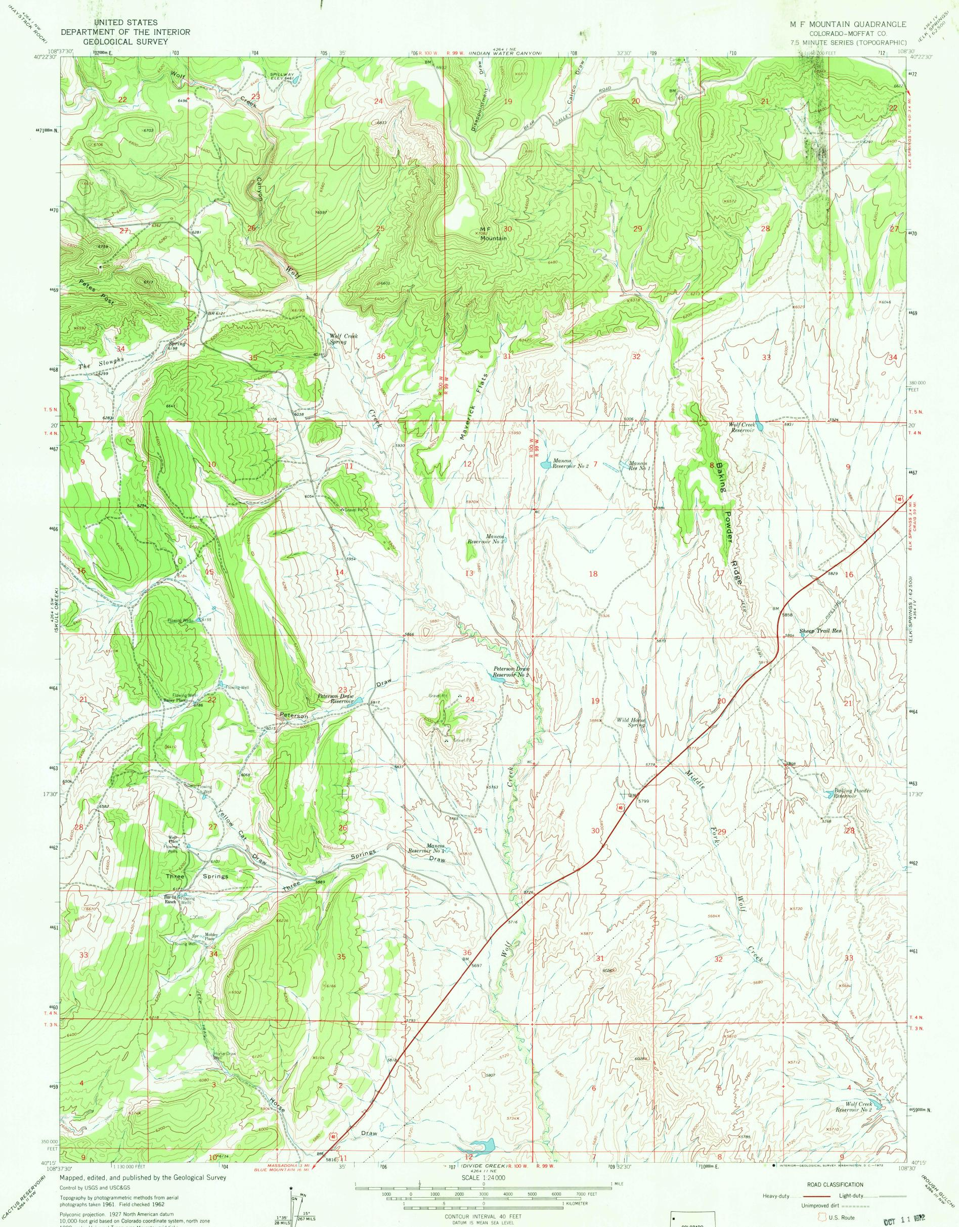
Polyconic projection. 1927 North American datum 10,000-foot grid based on Colorado coordinate system, north zone 1000-meter Universal Transverse Mercator grid ticks, zone 12, shown in blue
