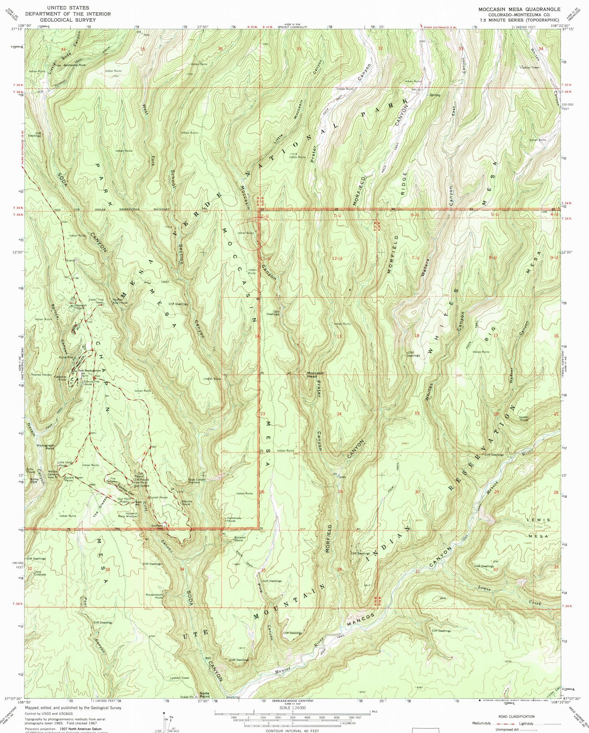
10,000-foot grid based on Colorado coordinate system, south zone 1000-meter Universal Transverse Mercator grid ticks, zone 12, shown in blue
