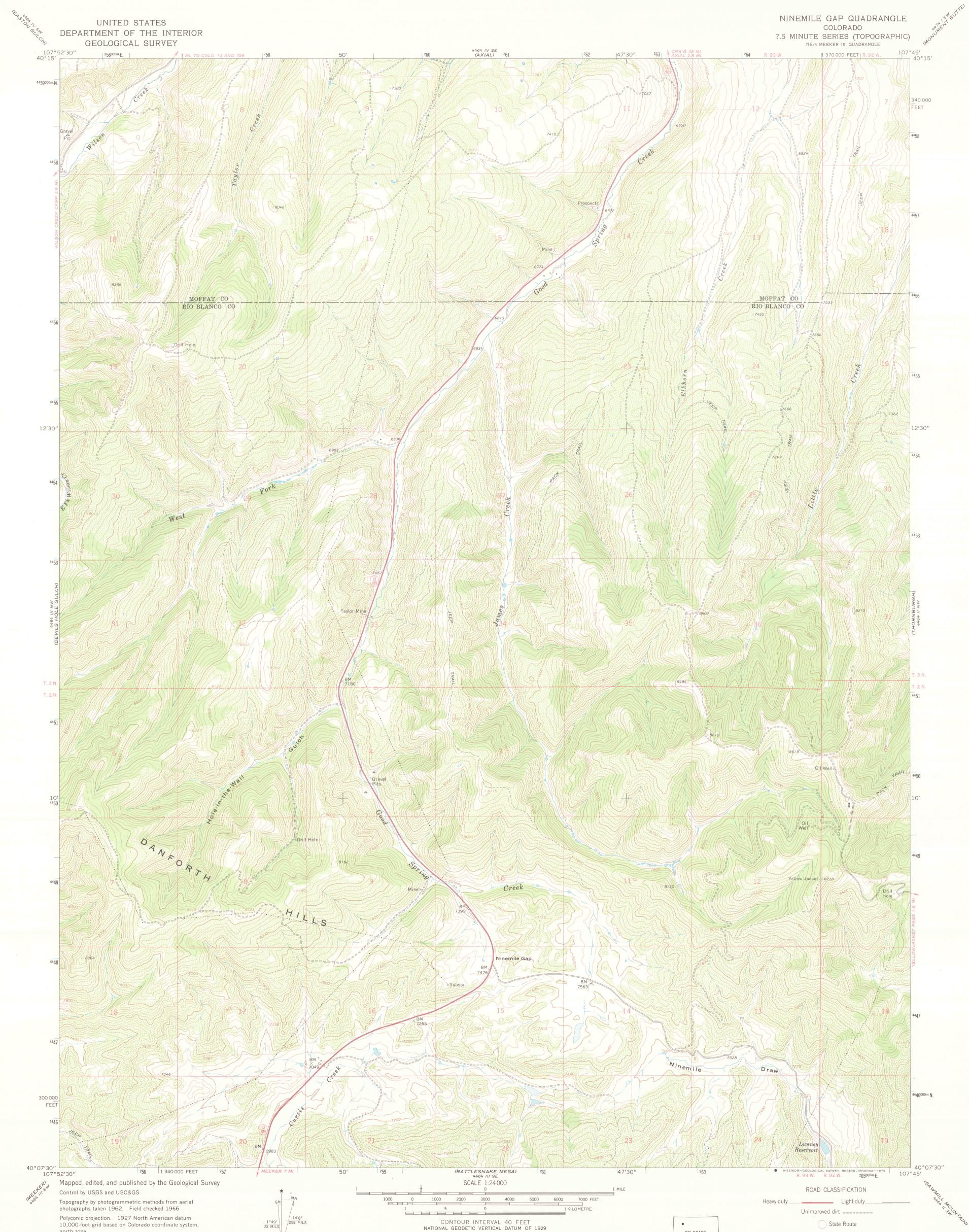
Polyconic projection. 1927 North American datum 10,000-foot grid based on Colorado coordinate system, north zone 1000-metre Universal Transverse Mercator grid ticks, zone 13, shown in blue
