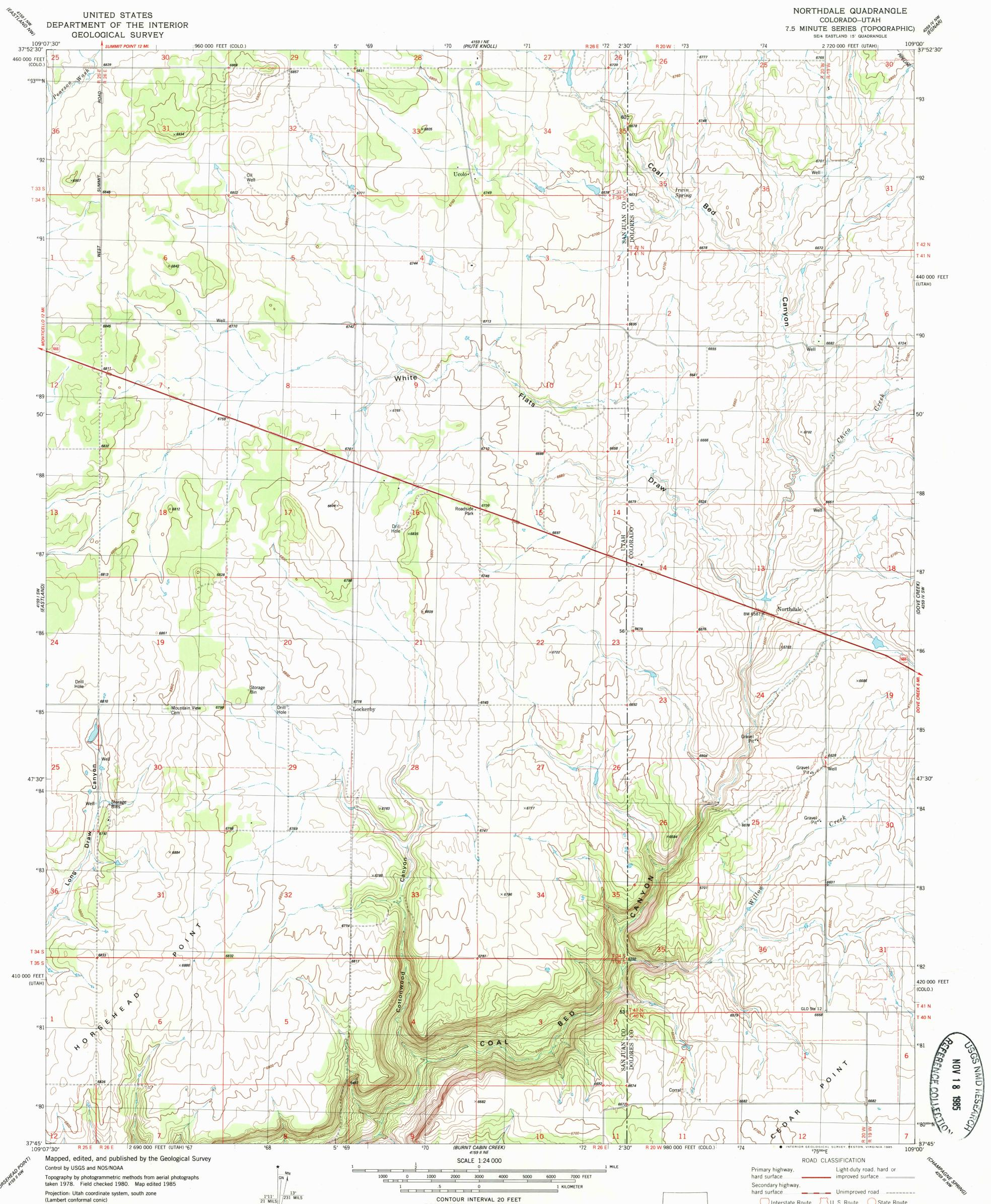
(Lambert conformal conic) 10,000-foot grid ticks based on Utah coordinate system, south zone and Colorado coordinate system, south zone 1000-meter Universal Transverse Mercator grid, zone 12 1927 North American Datum To place on the predicted North American Datum 1983 move the projection lines 4 meters north and 59 meters east as shown by dashed corner ticks Fine red dashed lines indicate selected fence lines
