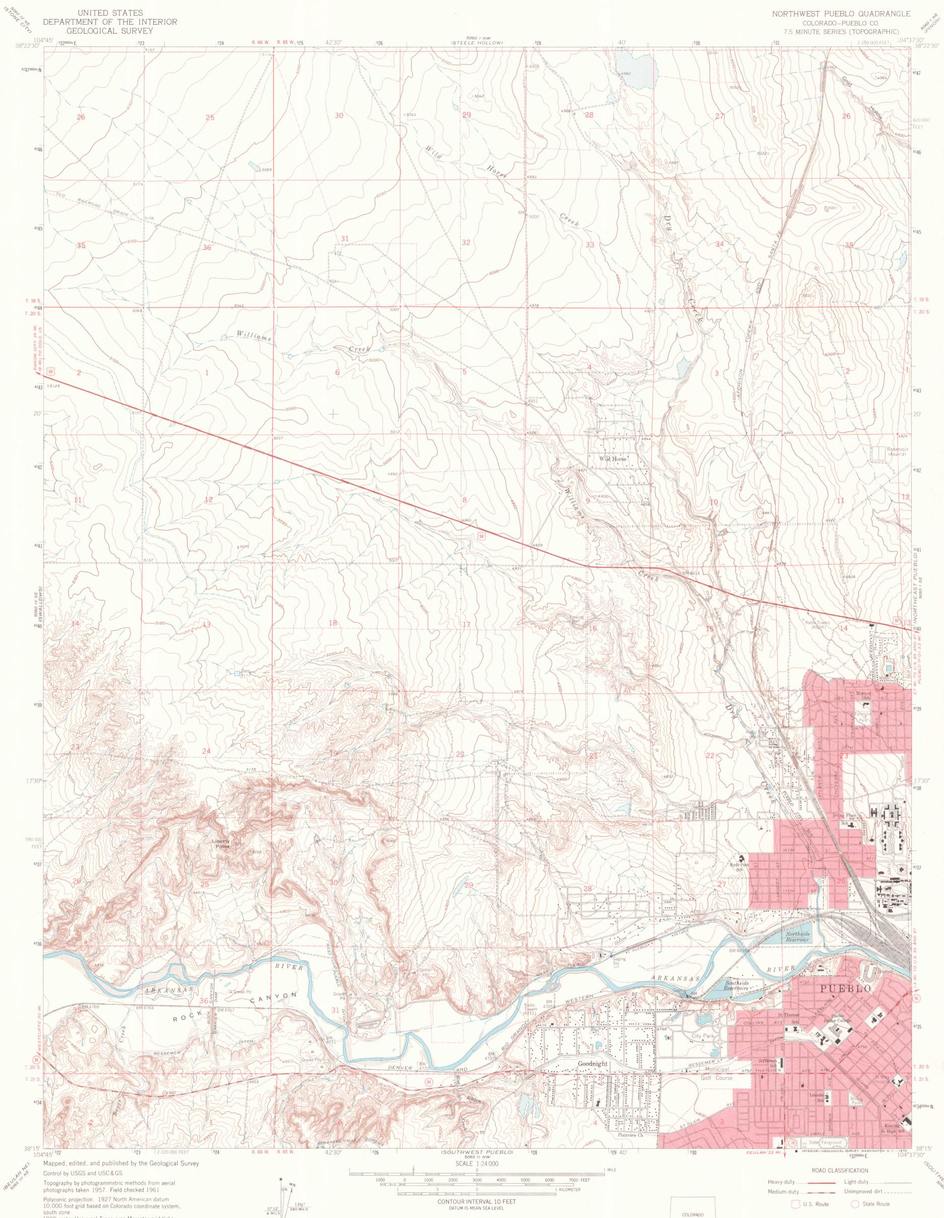
ction. 1927 North America 10,000-foot grid based on Colorado coordinate system, south zone 1000-meter Universal Transverse Mercator grid ticks, zone 13, shown in blue
