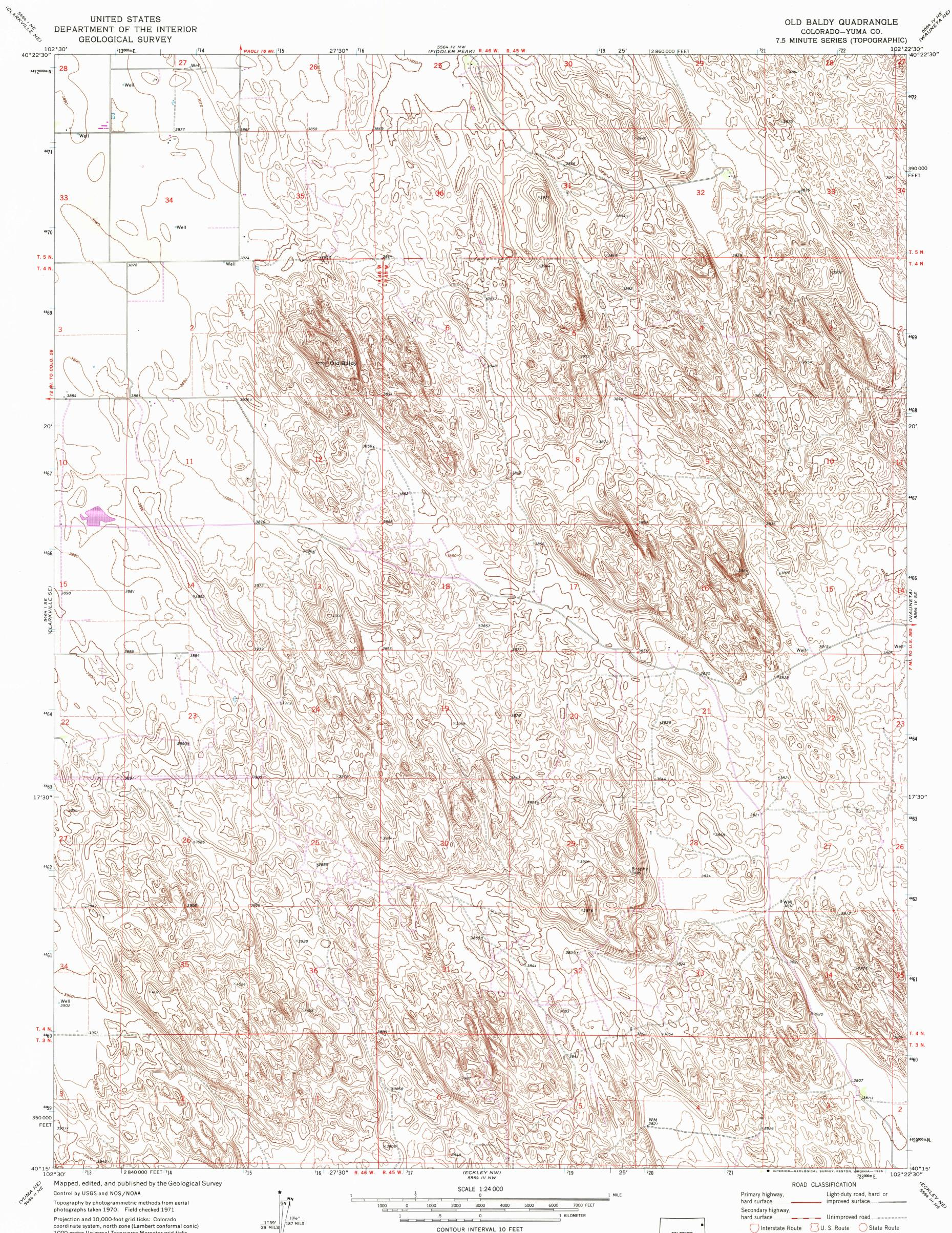
coordinate system, north zone (Lambert conformal conic) 1000-meter Universal Transverse Mercator grid ticks, zone 13, shown in blue. 1927 North American Datum Fine red dashed lines indicate selected fence lines To place on the predicted North American Datum 1983 move the projection lines 5 meters north and 41 meters east as shown by dashed corner ticks Revisions shown in purple compiled from aerial photographs taken 1980 and other source data. This information not field checked. Map edited 1984
