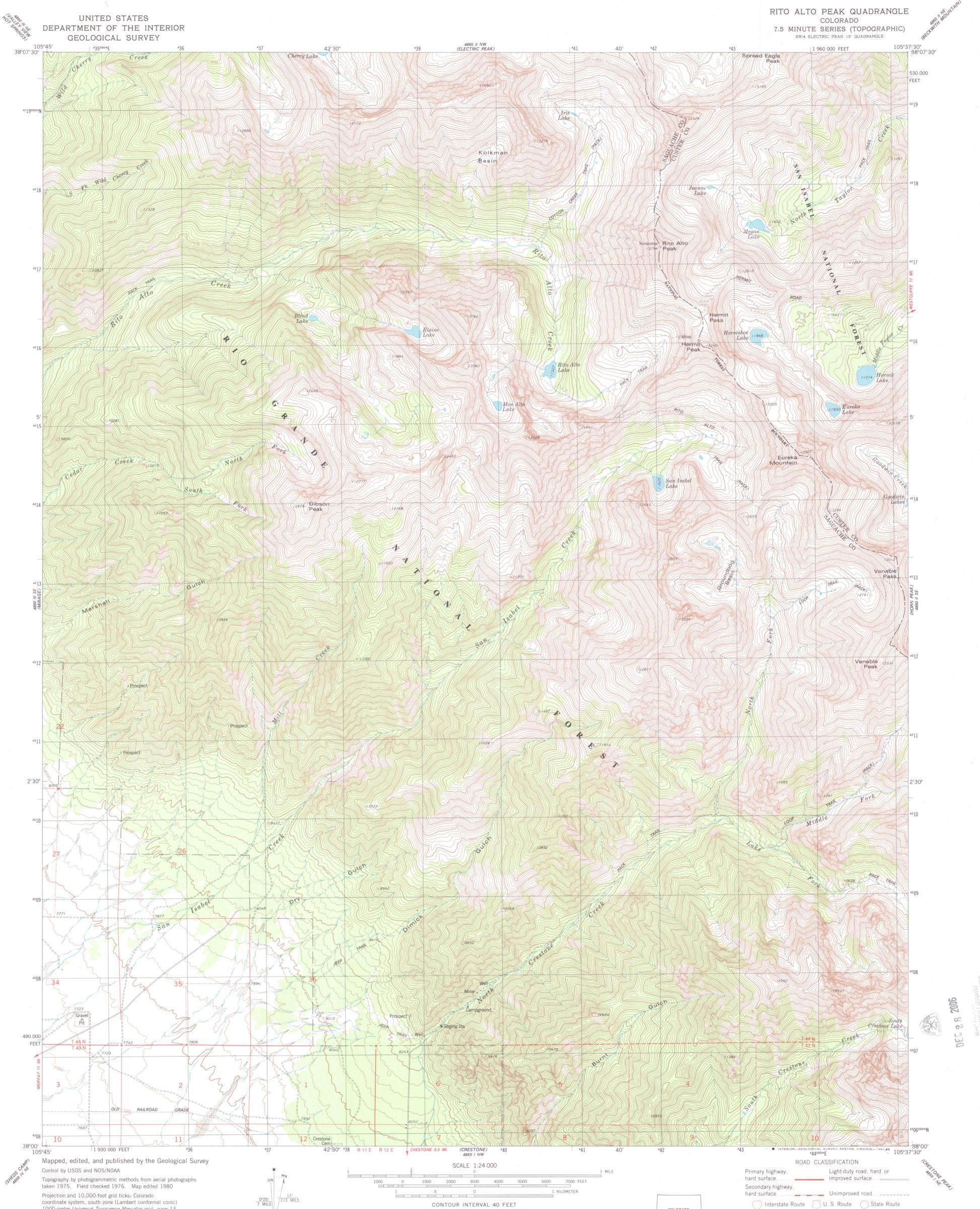
1000-meter Universal Transverse Mercator grid, zone 13 1927 North American datum To place on the predicted North American Datum 1983 move the projection lines 3 meters north and 50 meters east as shown by dashed corner ticks Fine red dashed lines indicate selected fence lines Certain land lines are omitted because of insufficient data There may be private inholdings within the boundaries of the National or State reservations shown on this map
