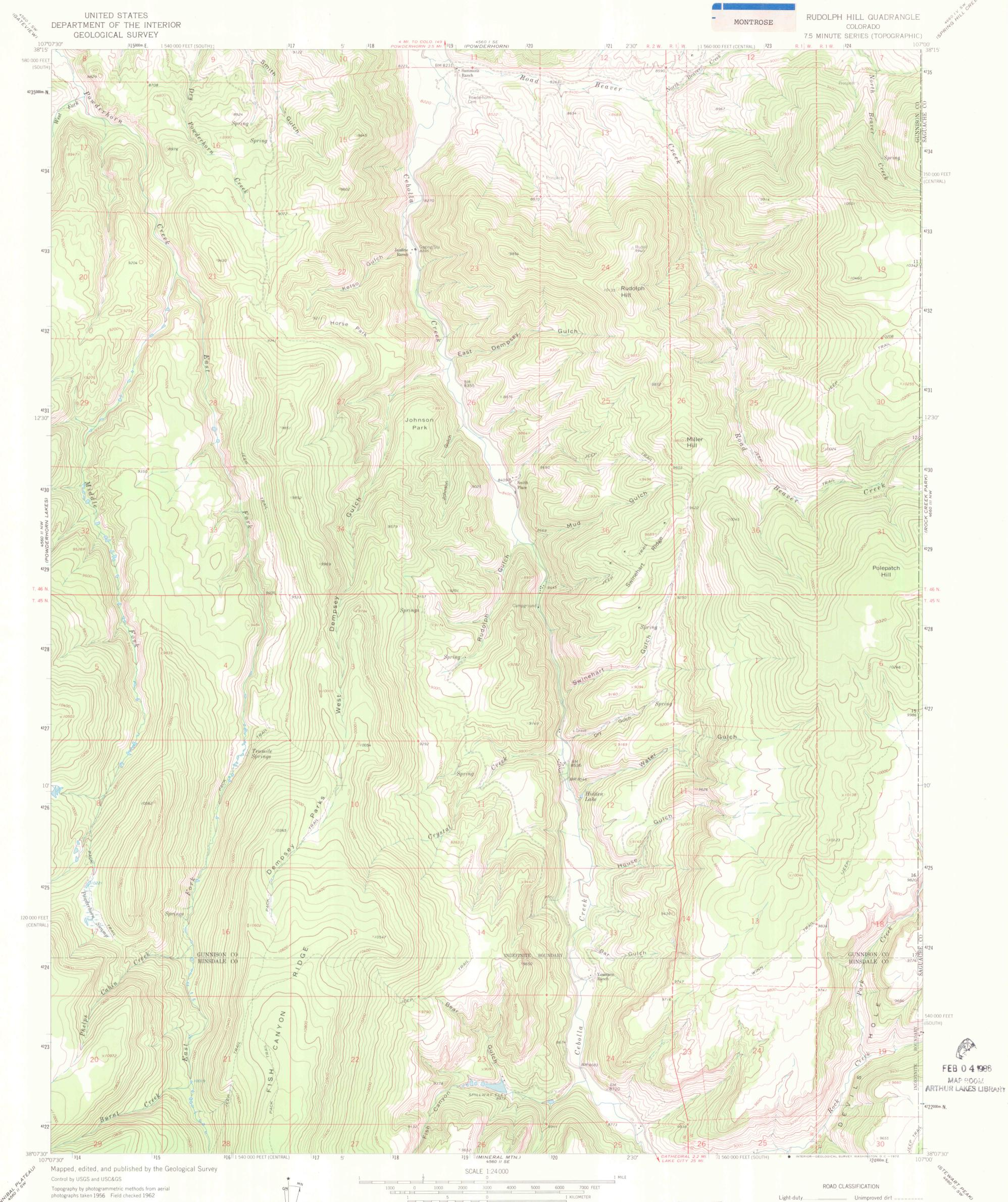
Polyconic projection. 1927 North American datum 10,000-foot grid based on Colorado coordinate system, central and south zones 1000-meter Universal Transverse Mercator grid ticks, zone 13, shown in blue
