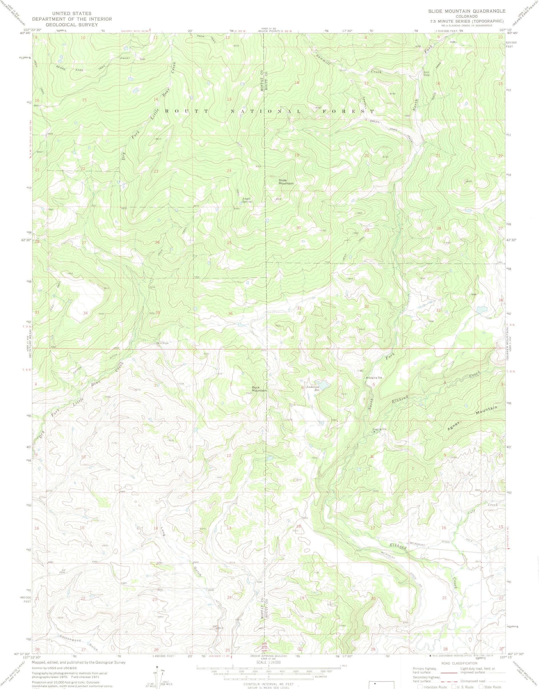
Projection and 10,000-foot grid ticks: Colorado coordinate system, north zone (Lambert conformal conic) 1000-meter Universal Transverse Mercator grid ticks, zone 13, shown in blue. 1927 North American datum
