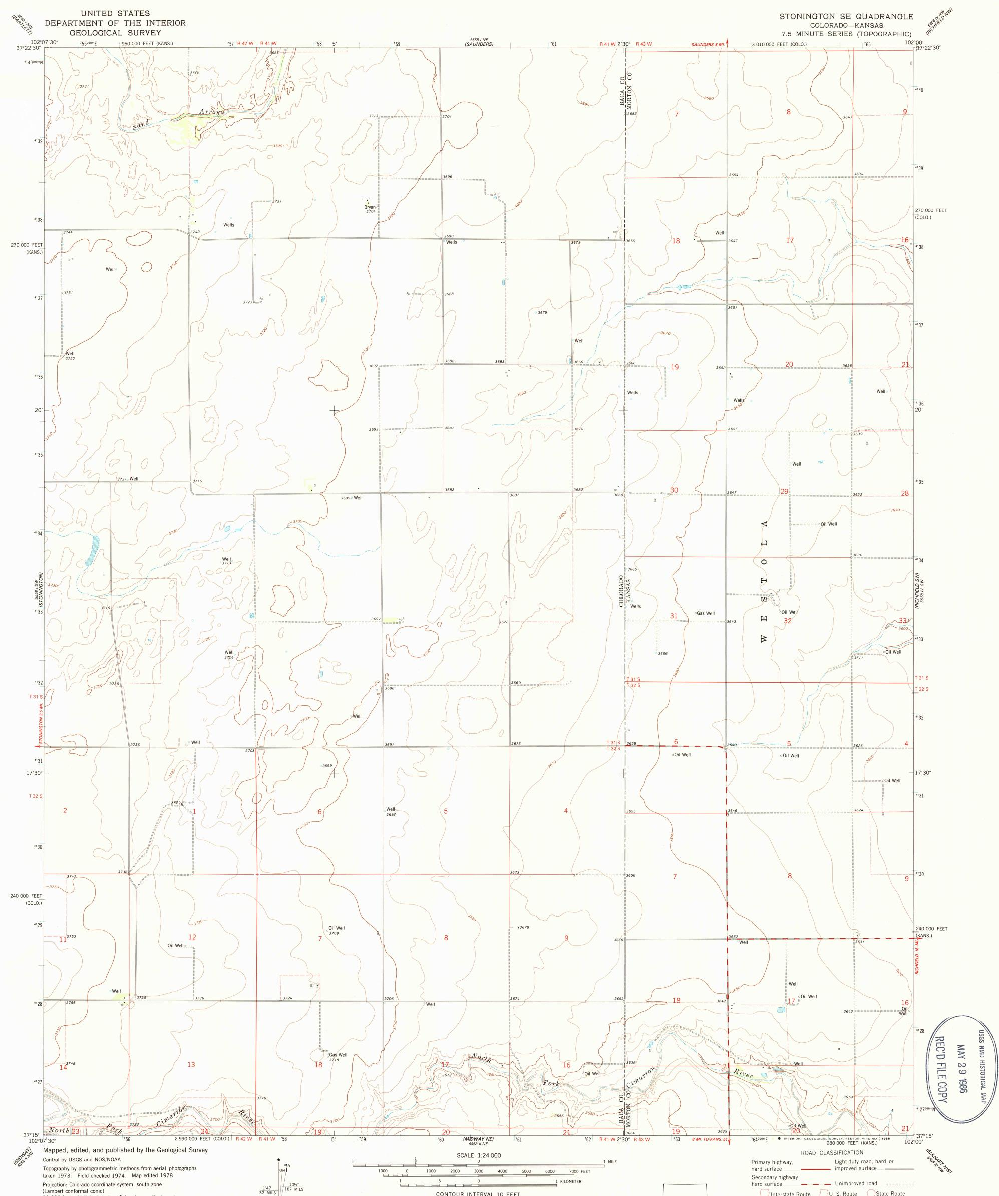
(Lambert conformal conic) 10,000-foot grid ticks based on Colorado coordinate system, south zone and Kansas coordinate system, south zone 1000-meter Universal Transverse Mercator grid ticks, zone 13, shown in blue. 1927 North American Datum Fine red dashed lines indicate selected fence lines
