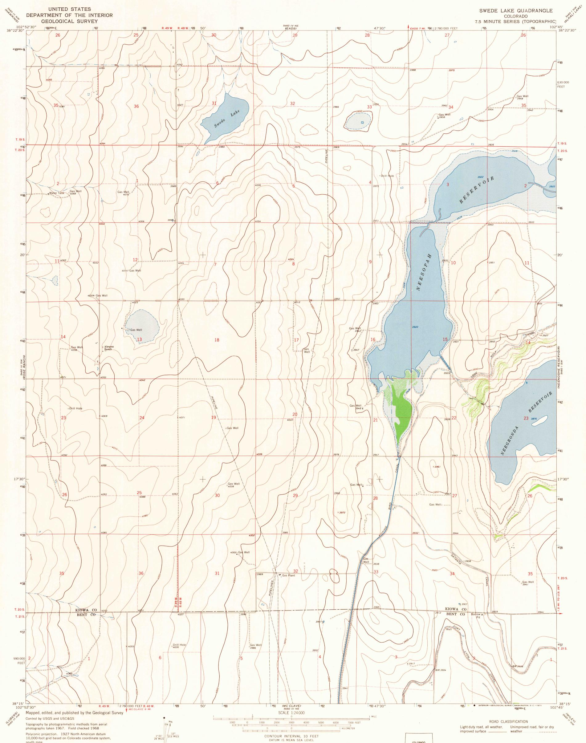
10,000-foot grid based on Colorado coordinate system, south zone 1000-meter Universal Transverse Mercator grid ticks, zone 13, shown in blue
