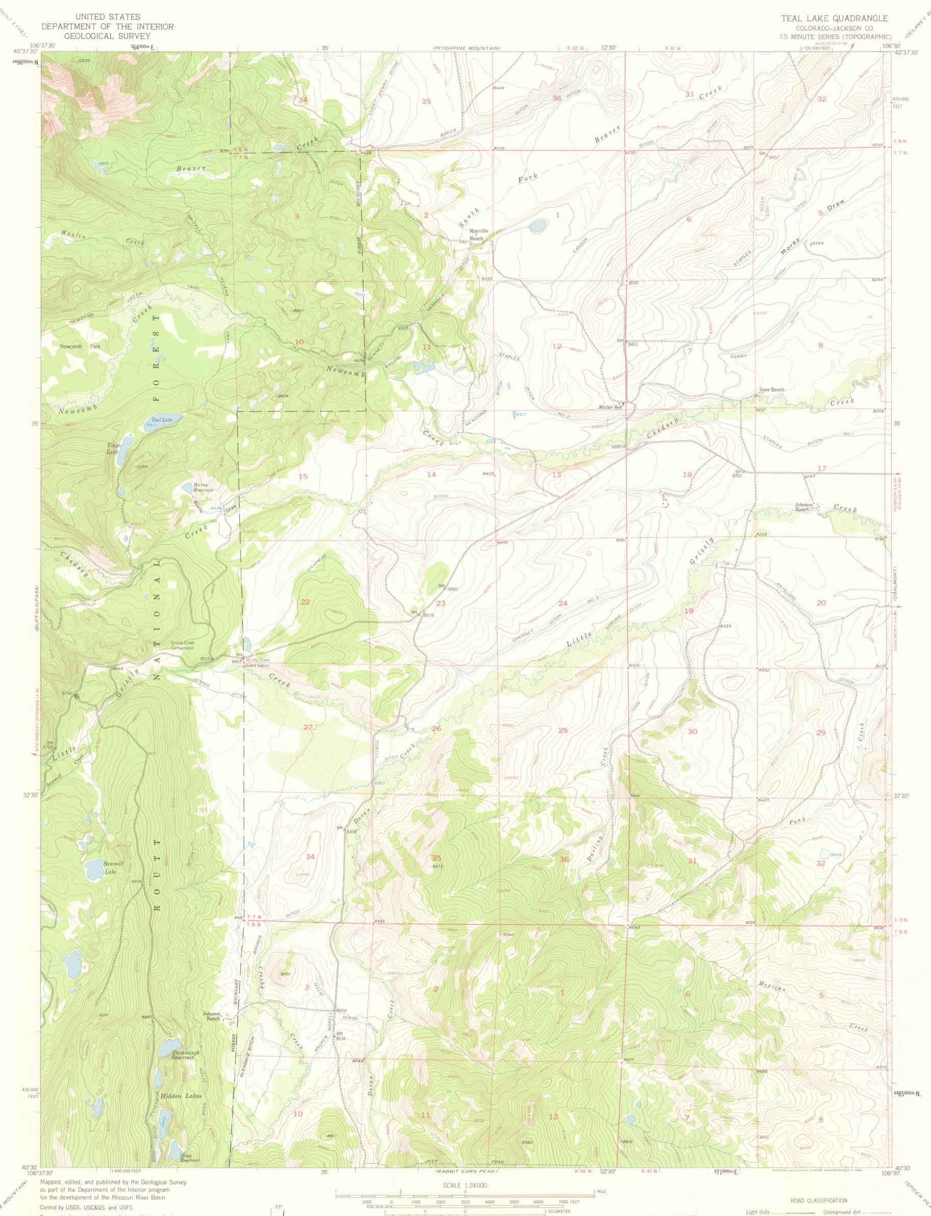
Topography from aerial photographs by multiplex methods Aerial photographs taken 1952. Field check 1955 Polyconic projection. 1927 North American datum 10,000-foot grid based on Colorado coordinate system, north zone 1000-meter Universal Transverse Mercator grid ticks, zone 13, shown in blue Dashed land lines indicate approximate locations Certain land lines are omitted in Ts. 6, 7 and 8 N.–R. 82 W. because of insufficient data Unchecked elevations are shown in brown
