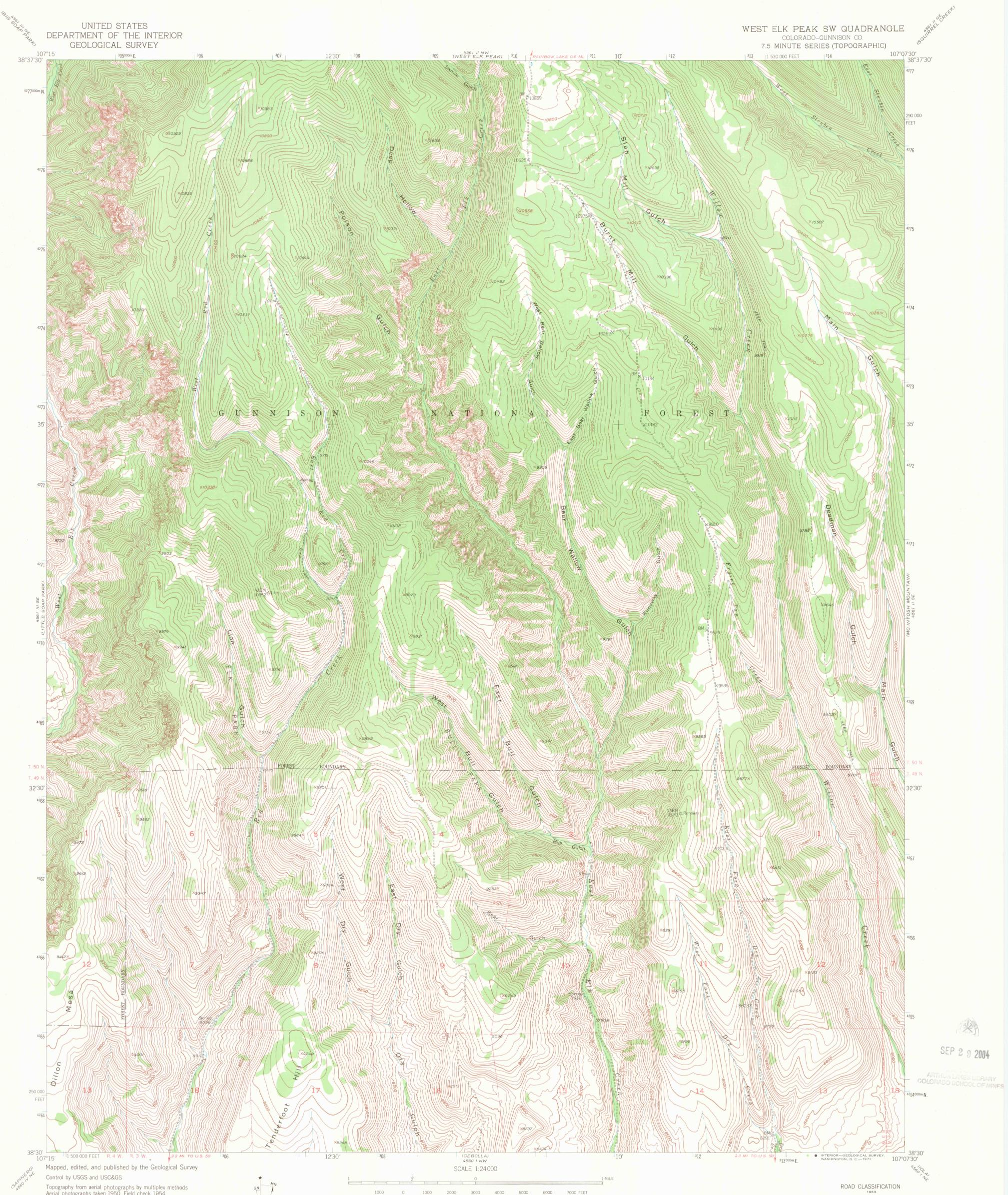
Aerial photographs taken 1950. Field check 1954 Polyconic projection. 1927 North American datum 10,000-foot grid based on Colorado coordinate system, central zone Dashed land lines indicate approximate locations Land lines omitted in T.50 N. Rs. 2, 3, and 4 W. because of insufficient data
