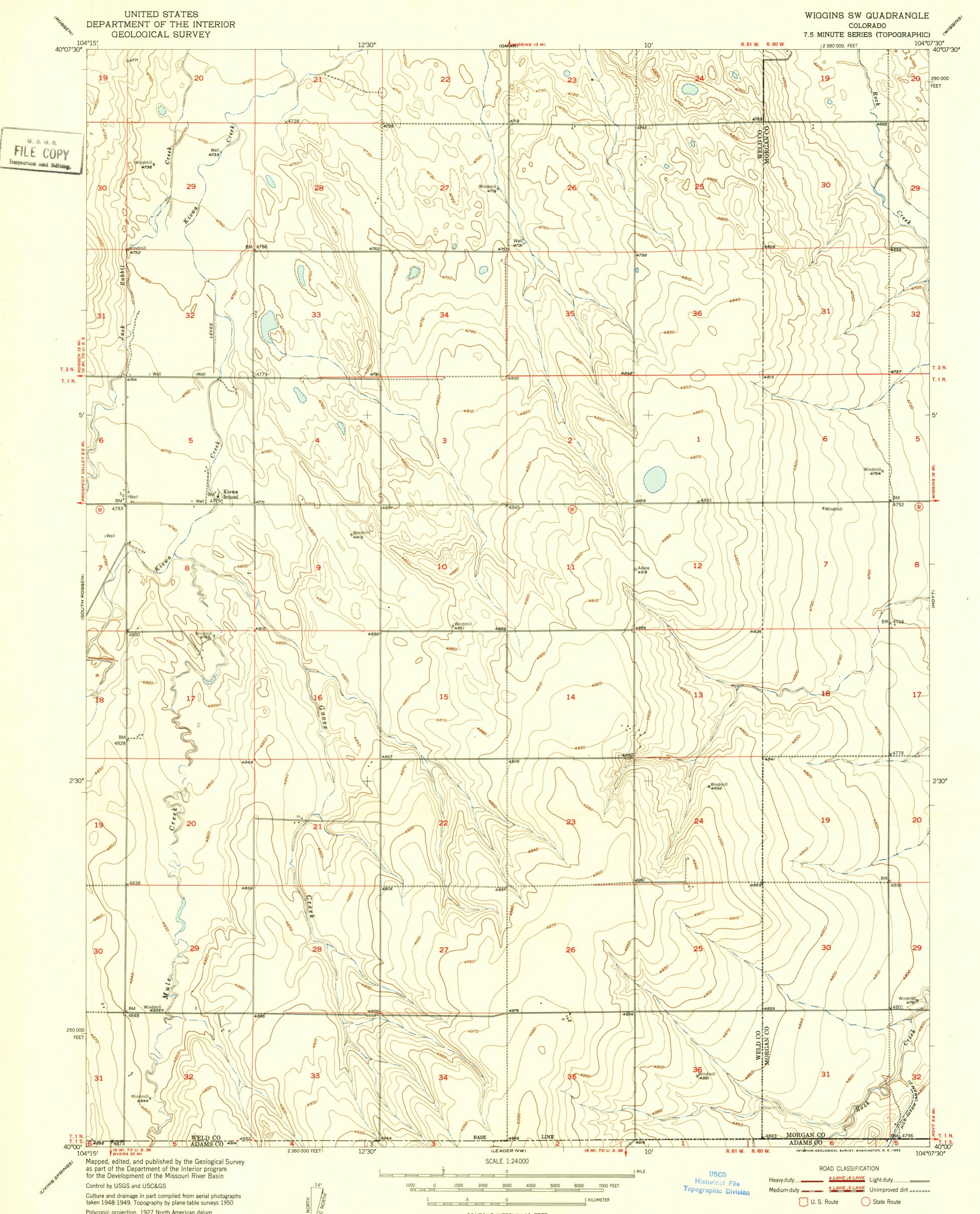
taken 1948-1949. Topography by plane-table surveys 1950 Polyconic projection. 1927 North American datum 10,000-foot grid based on Colorado coordinate system, north zone
