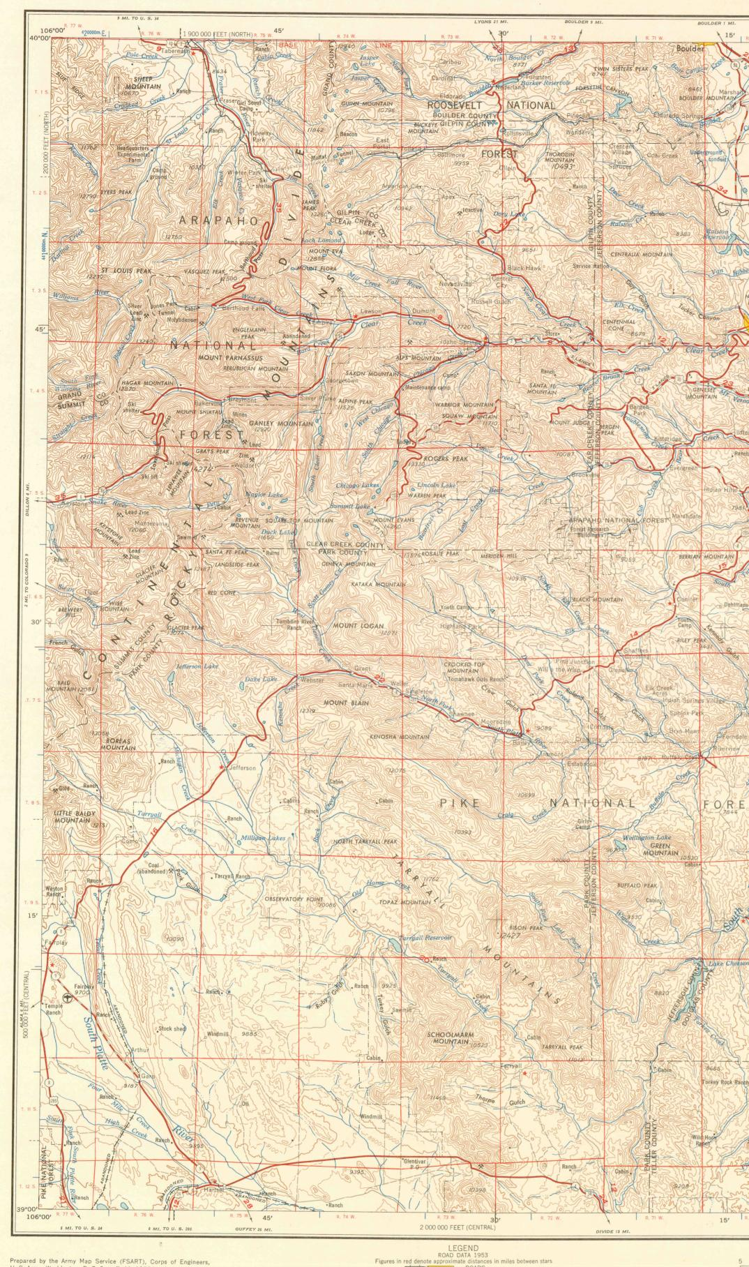
Prepared by the Army Map Service (FSART), Corps of Engineers, U. S. Army, Washington, D. C. Compiled in 1955 by photogrammetric methods and from: Colorado 1:24,000, USGS, 1937-53; Colorado 1:31,680, USGS, 1938-42; Colorado 1:62,500, USGS, 1903-40. Planimetric detail revised by photo-planimetric methods. Horizontal and Vertical Control by USC & GS, USGS, GLO, CE. Photography field annotated 1953.
