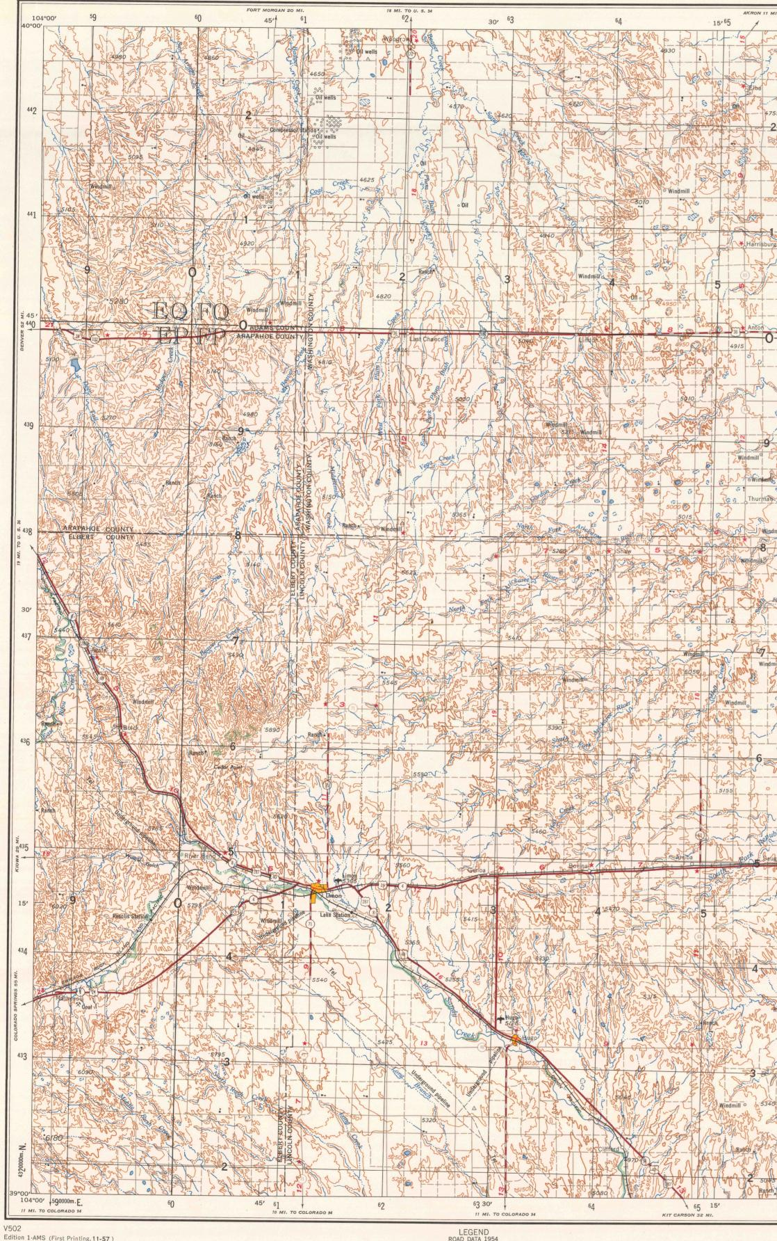
Edition 1-AMS (First Printing, 11-57) Prepared by the Army Map Service (BETT), Corps of Engineers, U. S. Army, Washington, D. C. Compiled in 1955 by photogrammetric methods. Horizontal and vertical control by USGS and USC&GS. Aerial photog-raphy 1953. Photography field annotated 1954.
