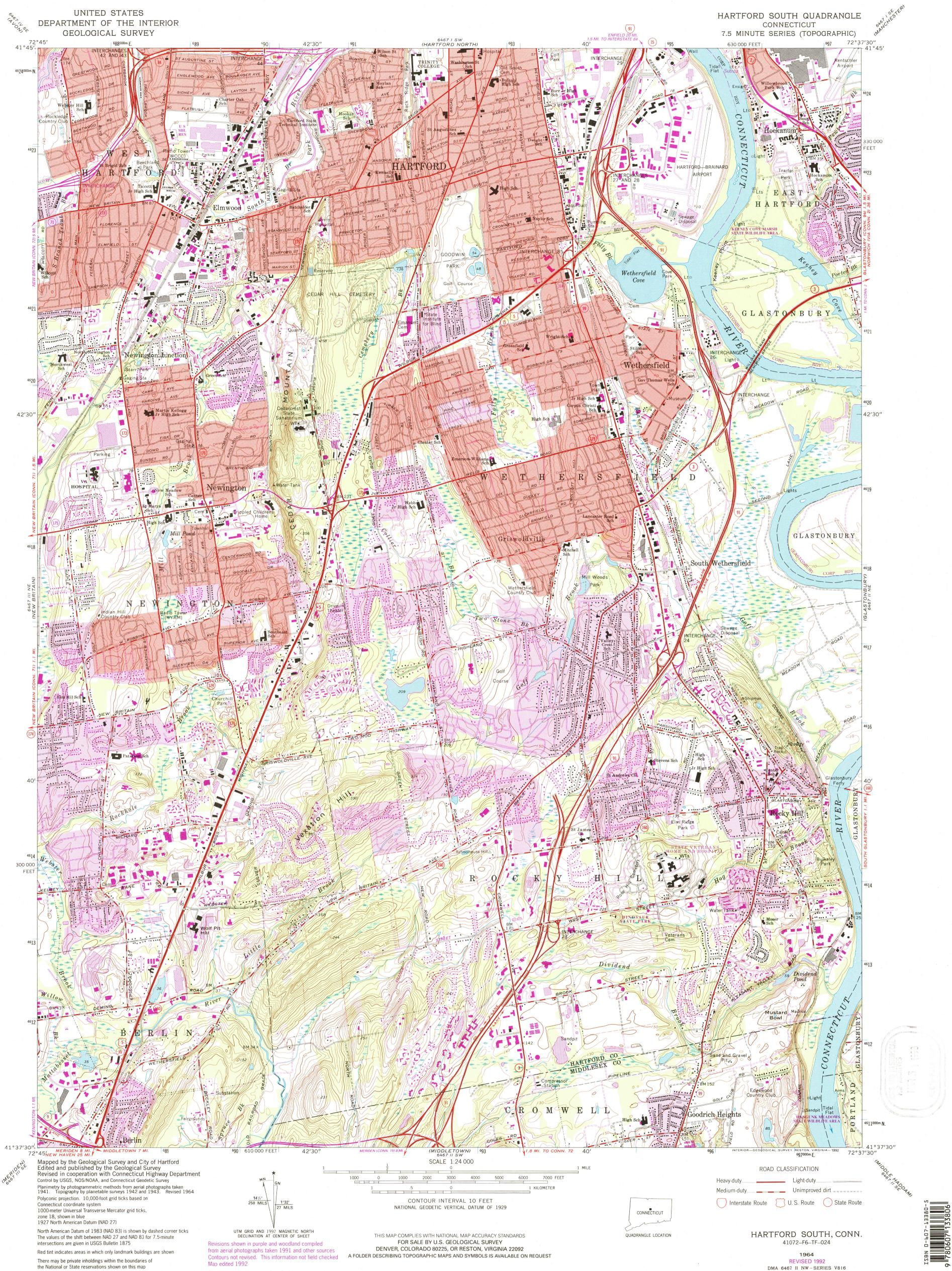
Connecticut coordinate system 1000-meter Universal Transverse Mercator grid ticks, zone 18, shown in blue 1927 North American Datum (NAD 27) North American Datum of 1983 (NAD 83) is shown by dashed corner ticks The values of the shift between NAD 27 and NAD 83 for 7.5-minute intersections are given in USGS Bulletin 1875
