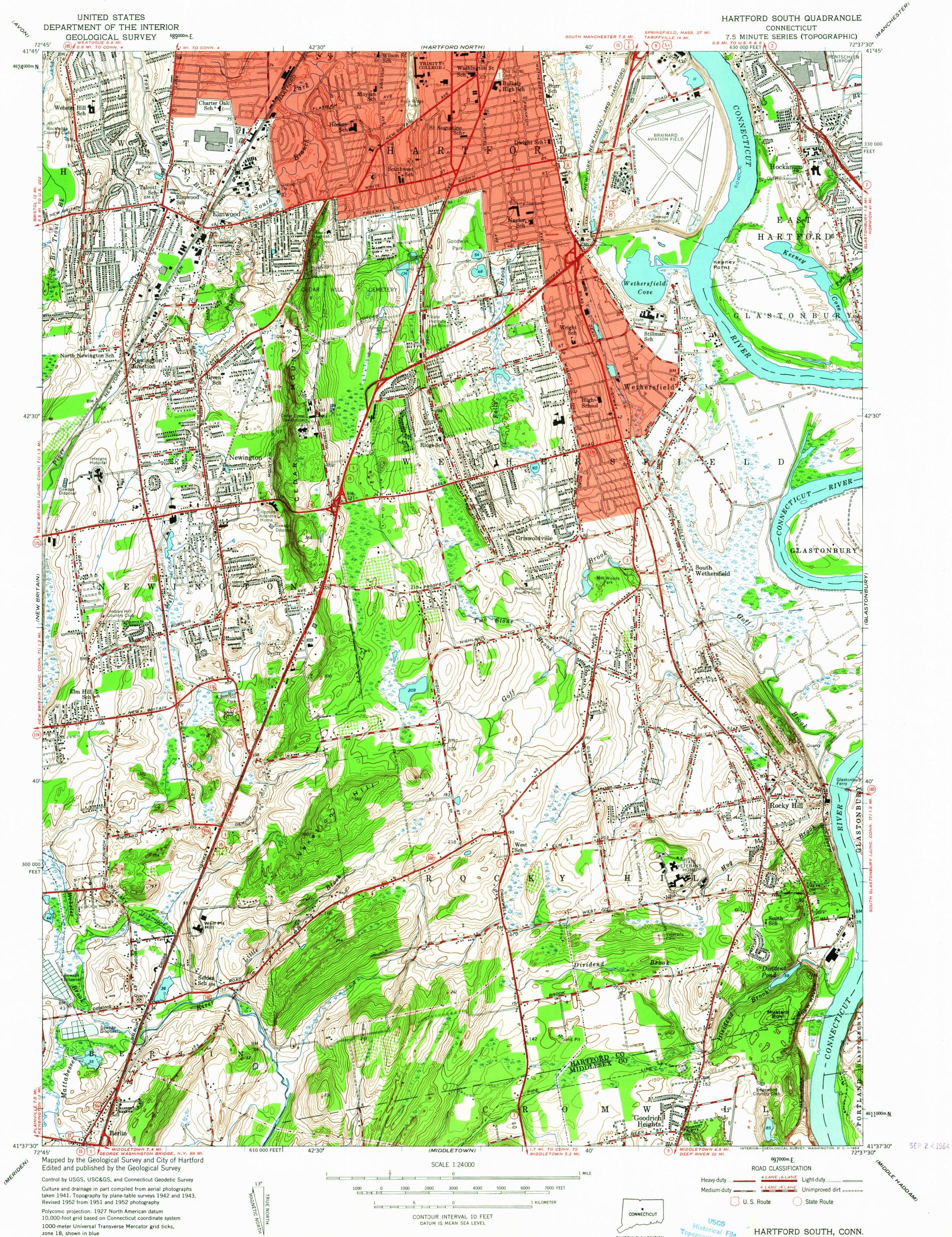
Polyconic projection. 1927 North American datum 10,000-foot grid based on Connecticut coordinate system 1000-meter Universal Transverse Mercator grid ticks, zone 18, shown in blue Red tint indicates areas in which only landmark buildings are shown
