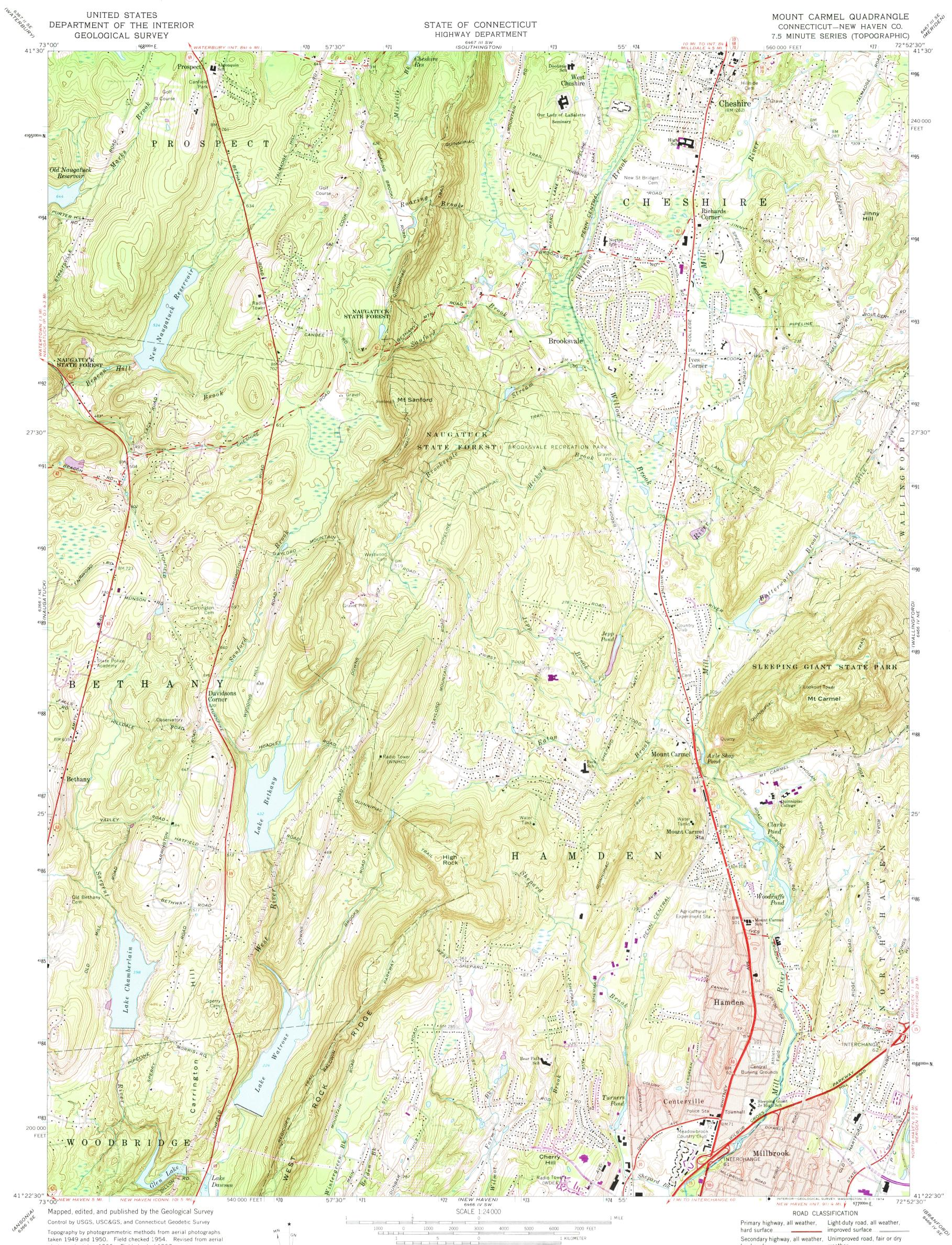
photographs taken 1966. Field checked 1967 Polyconic projection. 1927 North American datum 10,000-foot grid based on Connecticut coordinate system 1000-meter Universal Transverse Mercator grid ticks, zone 18, shown in blue
