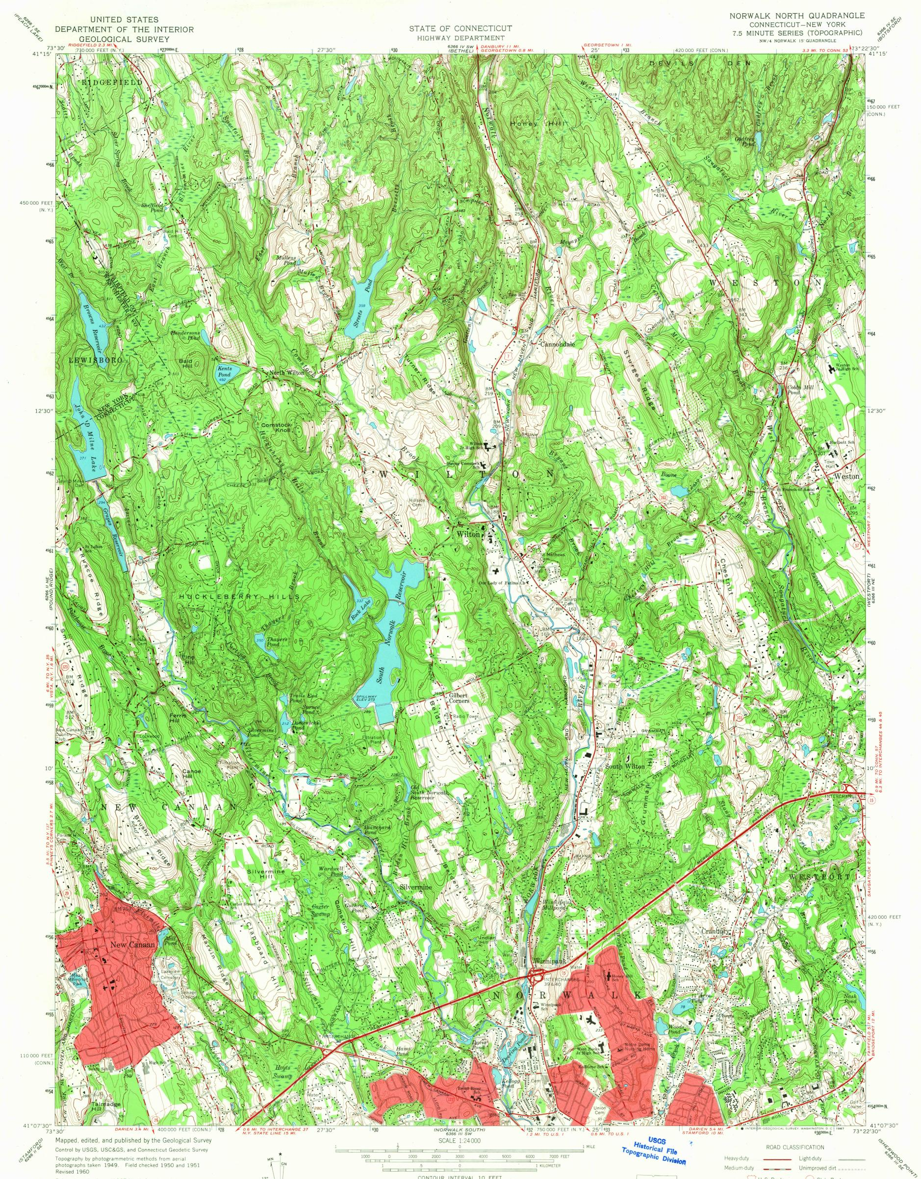
Polyconic projection. 1927 North American datum 10,000-foot grids based on Connecticut coordinate system, and New York coordinate system, east zone 1000-meter Universal Transverse Mercator grid ticks, zone 18, shown in blue
