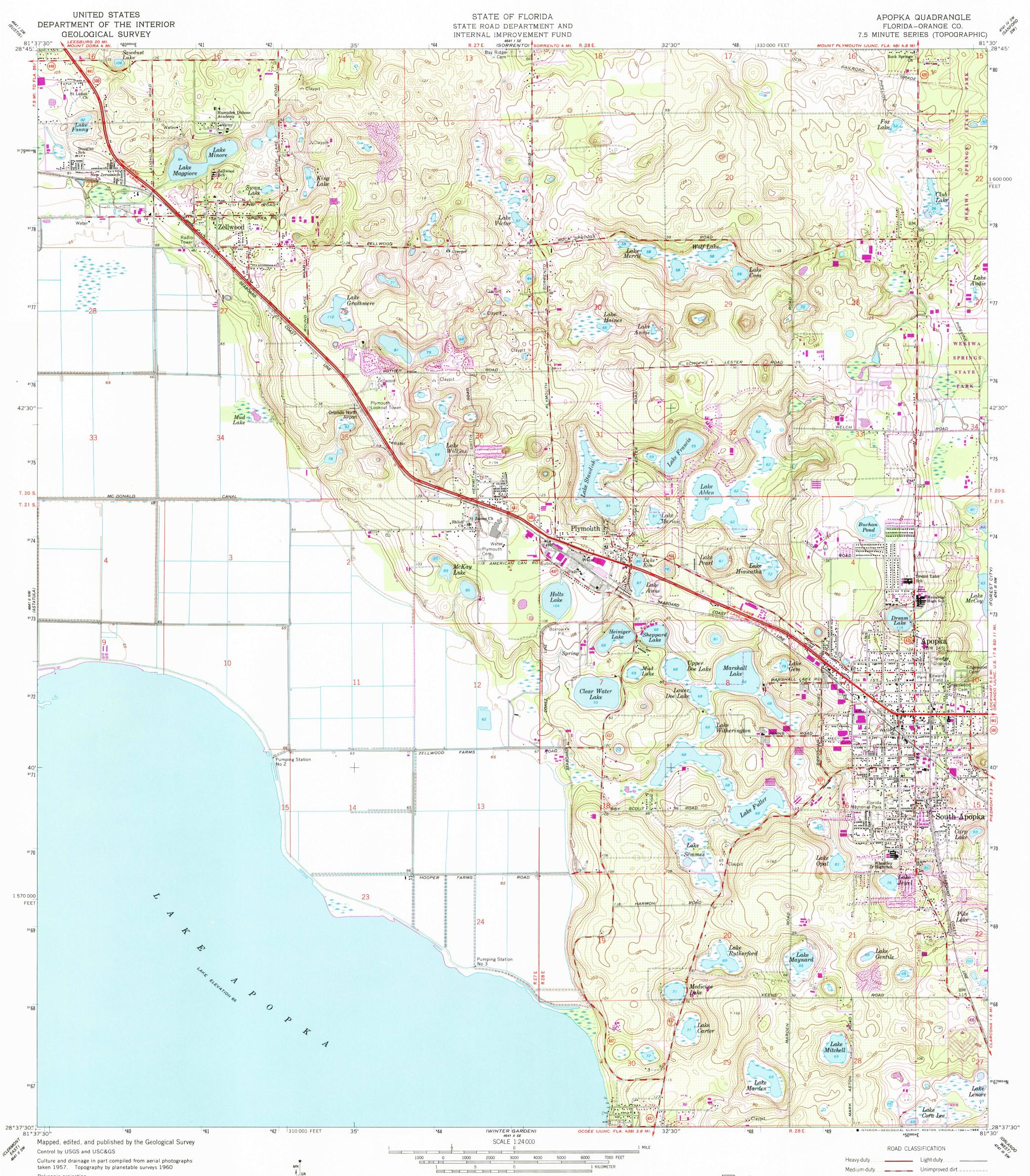
Polyconic projection 10,000-foot grid based on Florida coordinate system, east zone 1000-meter Universal Transverse Mercator grid ticks, zone 17, shown in blue. 1927 North American Datum To place on the predicted North American Datum 1983 move the projection lines 27 meters south and 18 meters west as shown by dashed corner ticks
