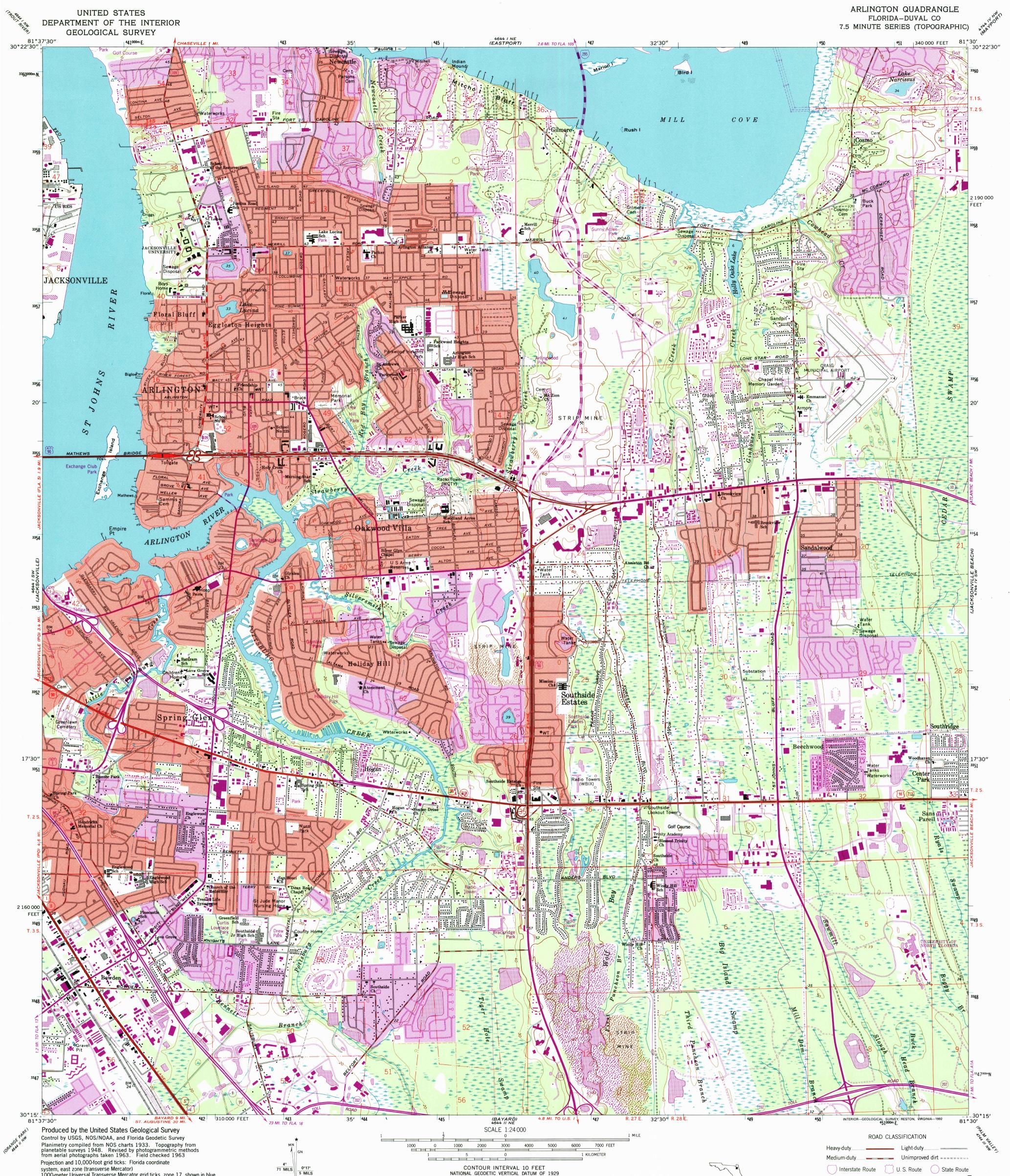
1000-meter Universal Transverse Mercator grid ticks, zone 17, shown in blue 1927 North American Datum (NAD 27) North American Datum of 1983 (NAD 83) is shown by dashed corner ticks The values of the shift between NAD 27 and NAD 83 for 7.5-minute intersections are given in USGS Bulletin 1875 Red tint indicates areas in which only landmark buildings are shown Fine red dashed lines indicate selected fence and field lines where generally visible on aerial photographs. This information is unchecked
