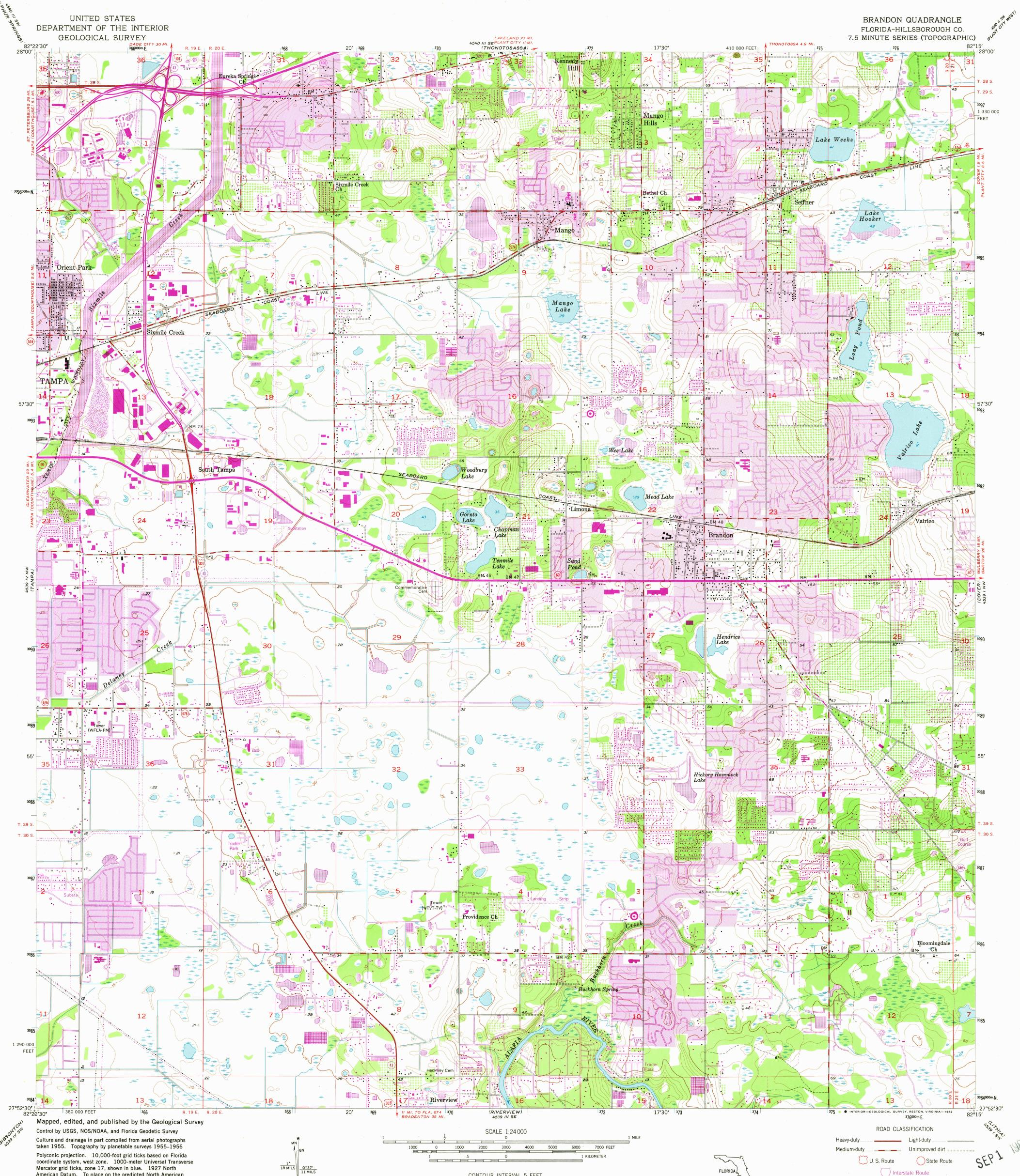
Mercator grid ticks, zone 17, shown in blue. 1927 North American Datum. To place on the predicted North American Datum 1983 move the projection lines 29 meters south and 17 meters west as shown by dashed corner ticks
