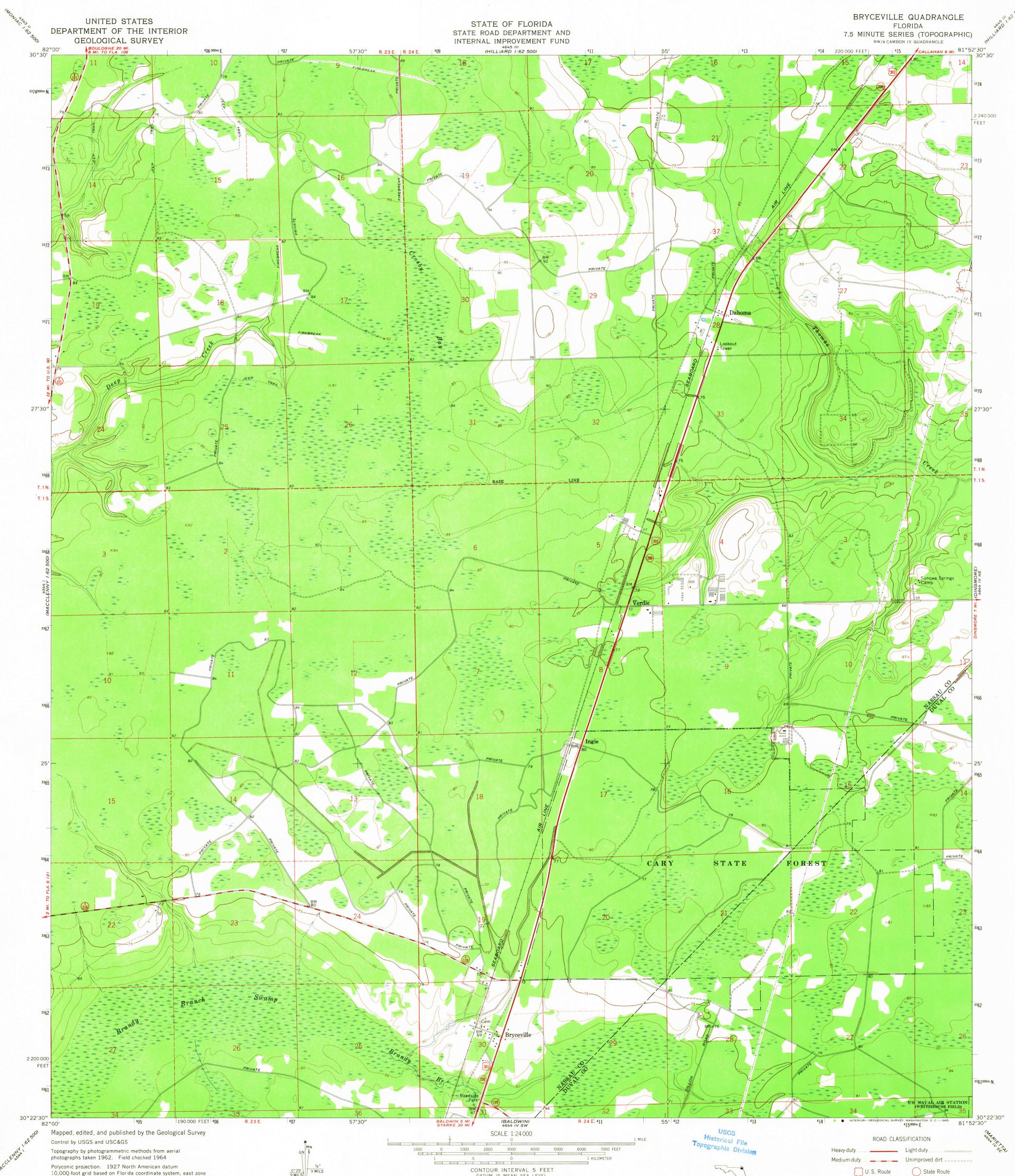
Polyconic projection. 1927 North American datum 10,000-foot grid based on Florida coordinate system, east zone 1000-meter Universal Transverse Mercator grid ticks, zone 17, shown in blue
