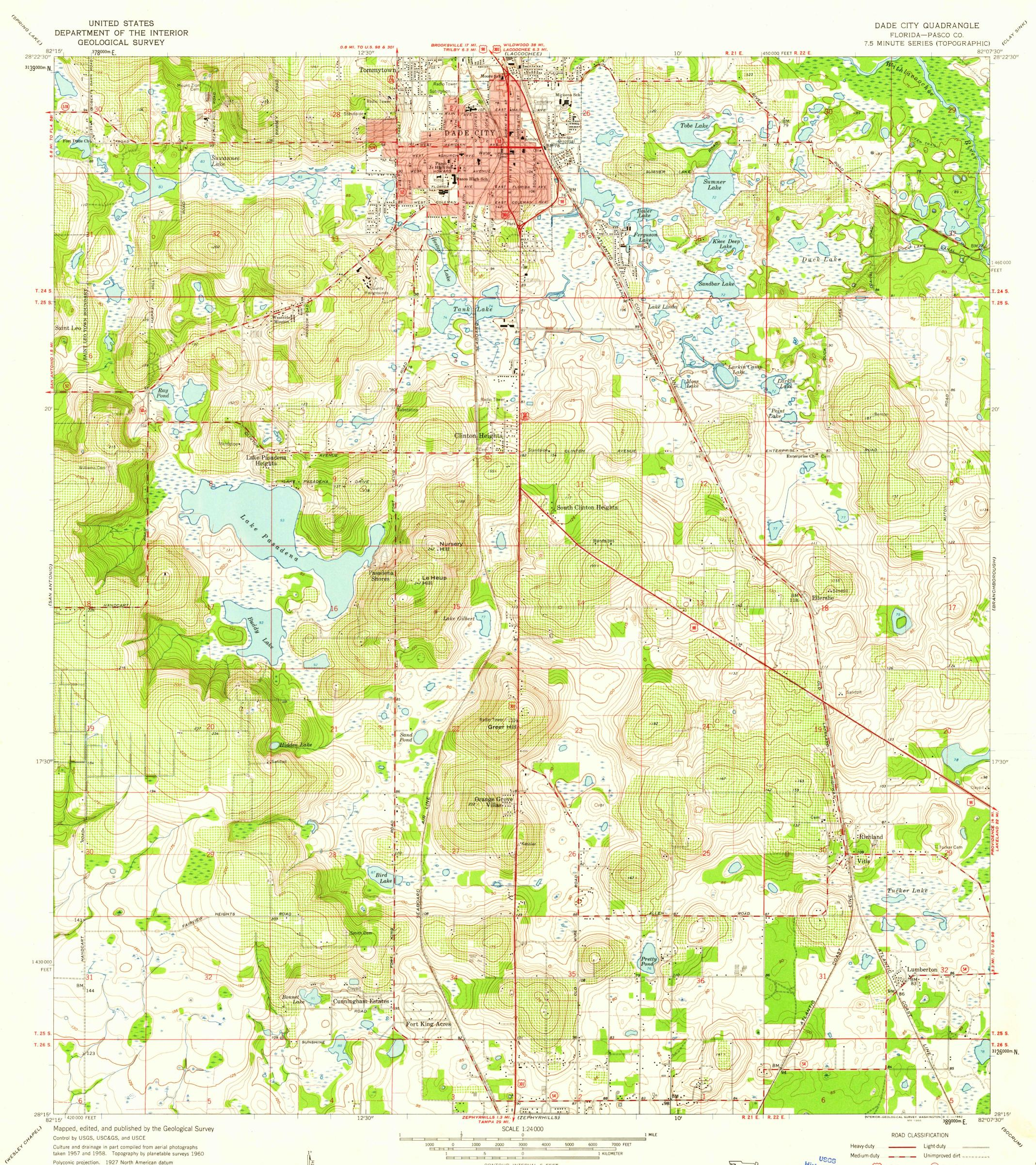
taken 1957 and 1958. Topography by planetable surveys 1960 Polyconic projection. 1927 North American datum 10,000-foot grid based on Florida coordinate system, west zone 1000-meter Universal Transverse Mercator grid ticks, zone 17, shown in blue Fine red dashed lines indicate selected fence and field lines where generally visible on aerial photographs. This information is unchecked Red tint indicates area in which only landmark buildings are shown
