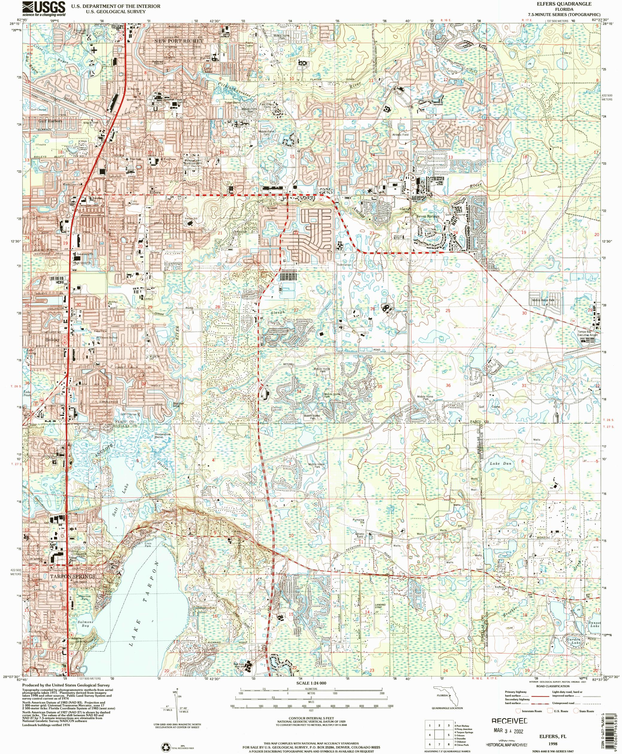
North American Datum of 1927 (NAD 27) is shown by dashed corner ticks. The values of the shift between NAD 83 and NAD 27 for 7.5-minute intersections are obtainable from National Geodetic Survey NADCON software Landmark buildings verified 1974
