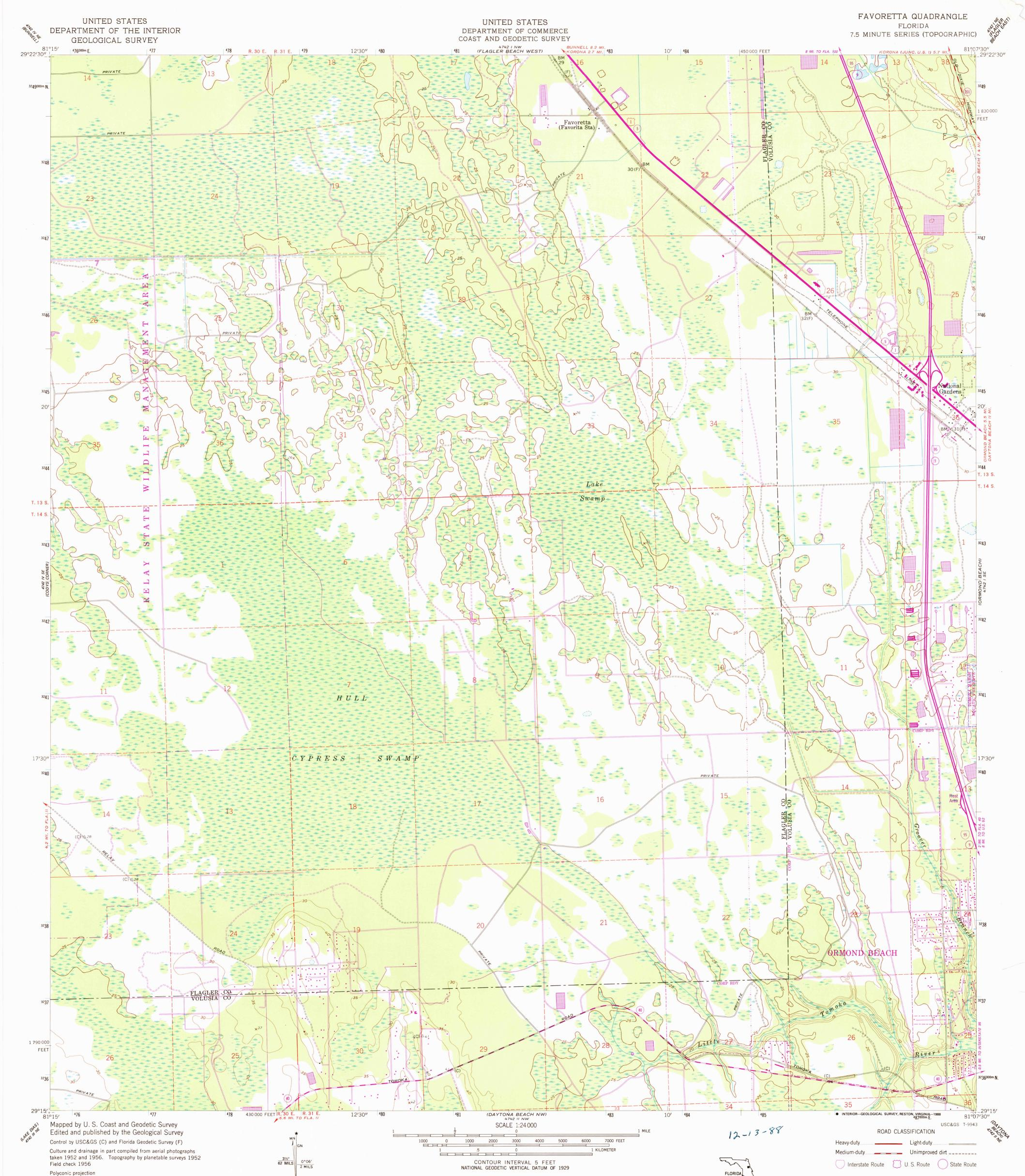
Polyconic projection 10,000-foot grid based on Florida coordinate system, east zone 1000-meter Universal Transverse Mercator grid ticks, zone 17, shown in blue. 1927 North American Datum To place on the predicted North American Datum 1983, move the projection lines 25 meters south and 18 meters west as shown by dashed corner ticks
