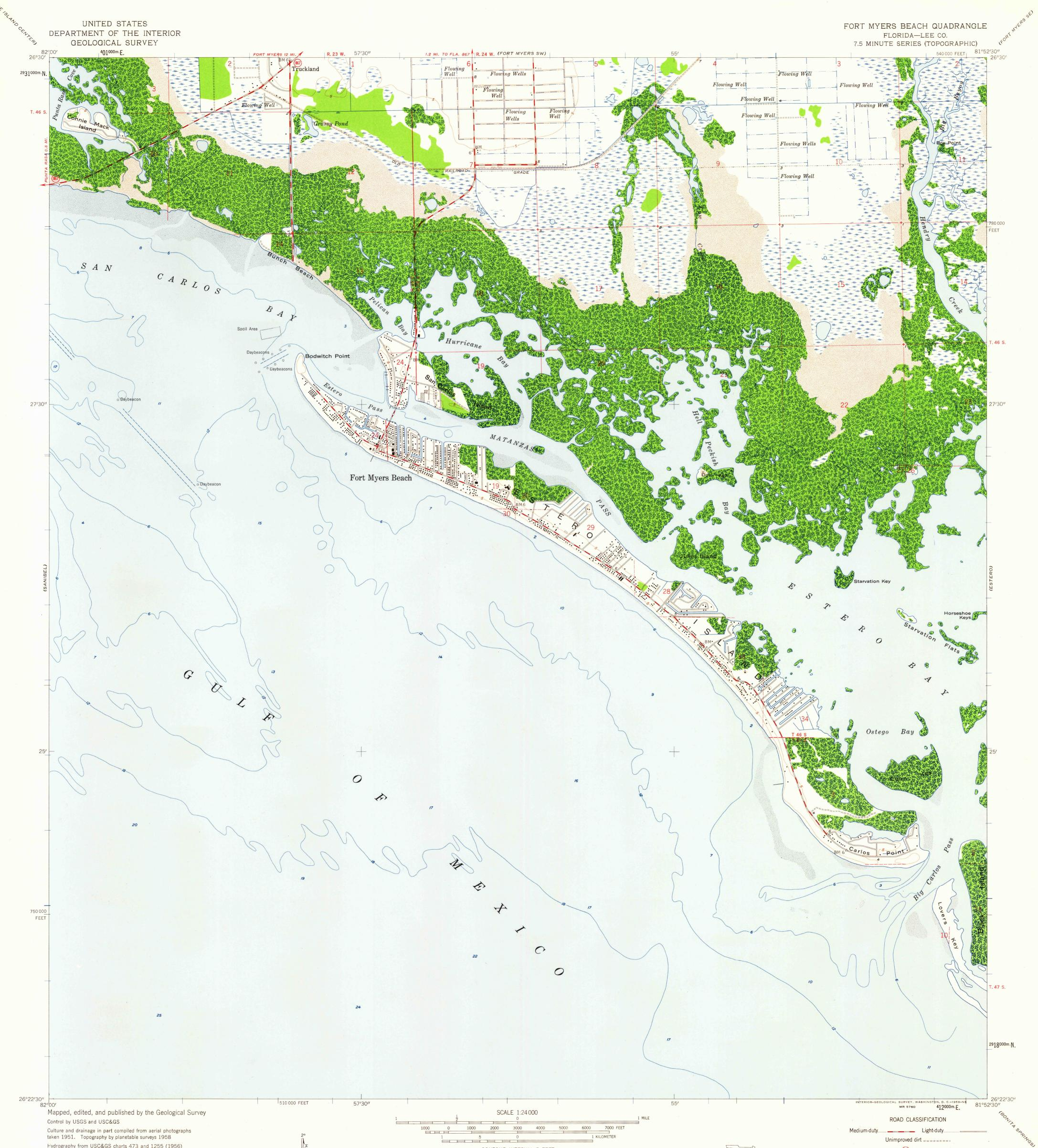
Hydrography from USC&GS charts 473 and 1255 (1956) Polyconic projection. 1927 North American datum 10,000-foot grid based on Florida coordinate system, west zone 1000-meter Universal Transverse Mercator grid ticks, zone 17, shown in blue
