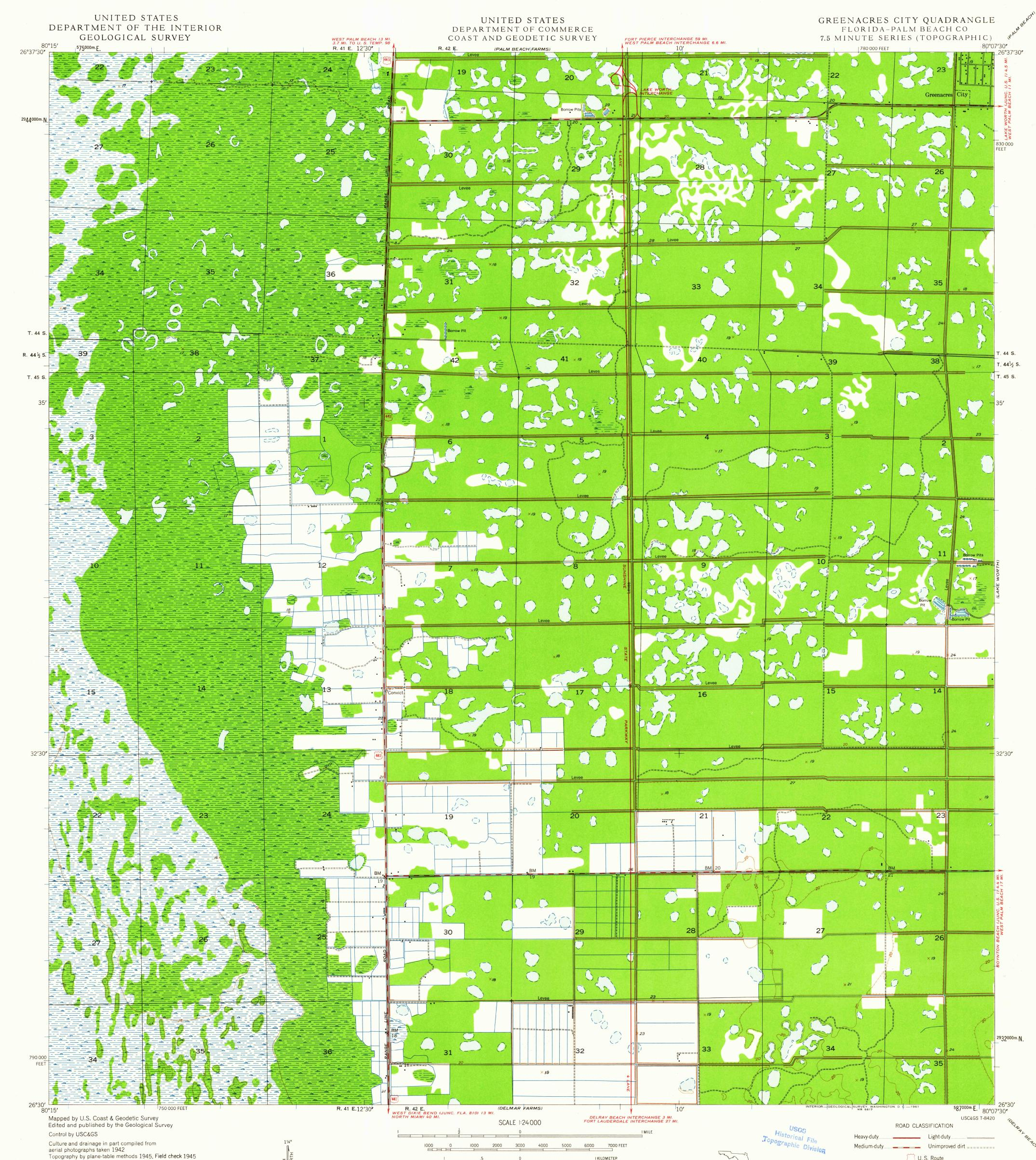
Polyconic projection. 1927 North American datum 10,000-foot grid based on Florida coordinate system, east zone 1000-meter Universal Transverse Mercator grid ticks, zone 17, shown in blue
