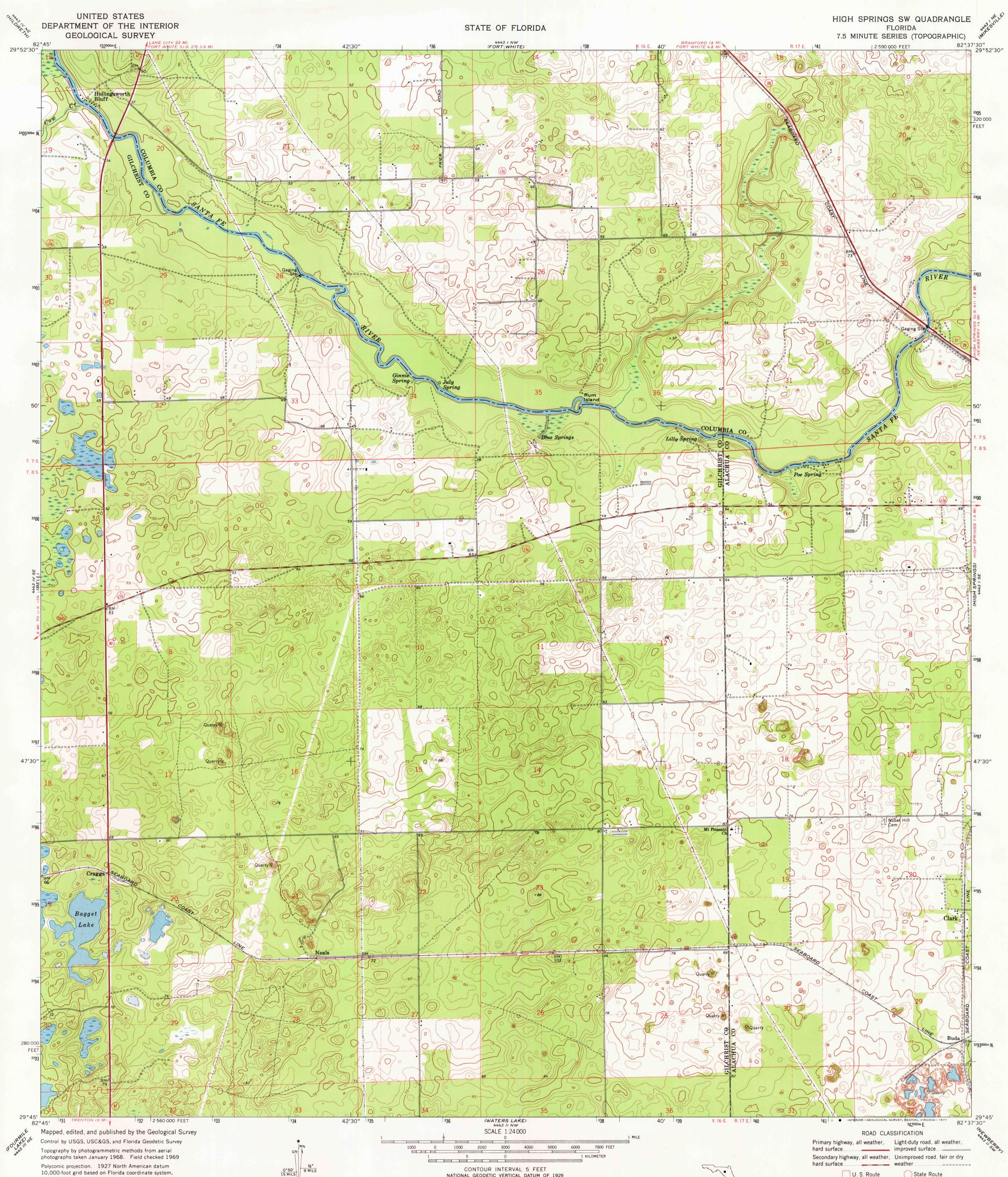
Polyconic projection. 1927 North American datum 10,000-foot grid based on Florida coordinate system, north zone 1000-meter Universal Transverse Mercator grid ticks, zone 17, shown in blue
