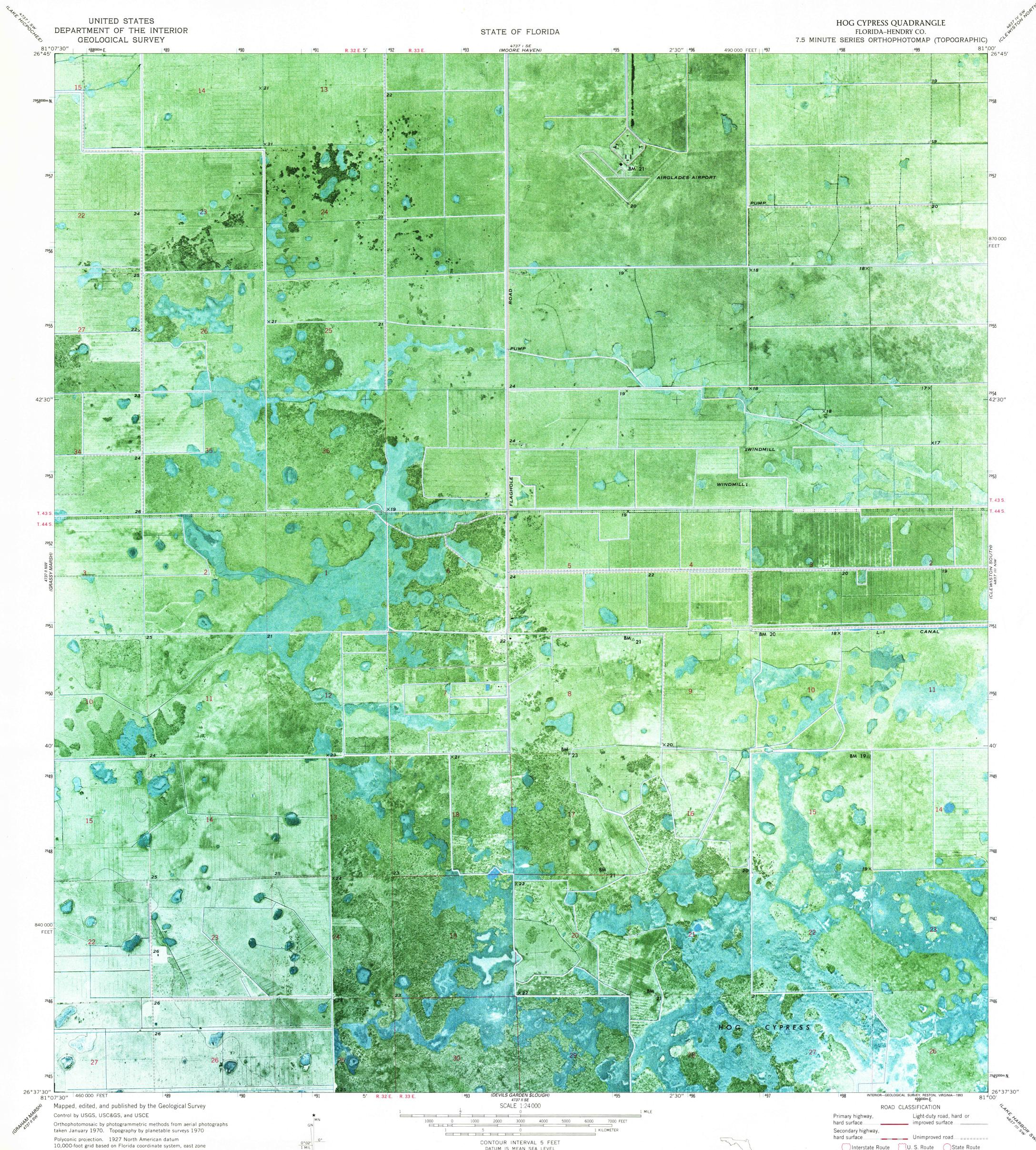
10,000-foot grid based on Florida coordinate system, east zone 1000-meter Universal Transverse Mercator grid ticks, zone 17, shown in blue
