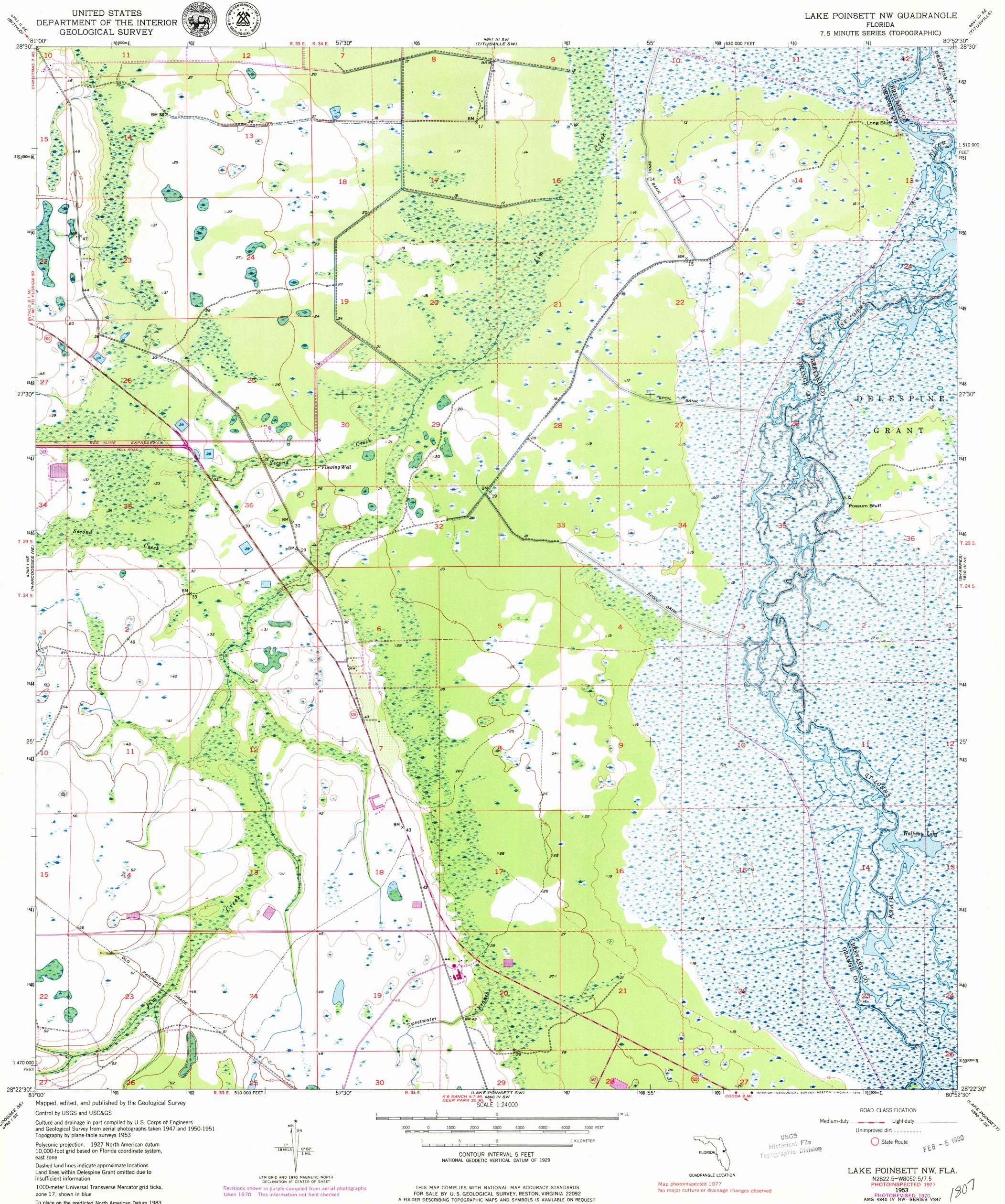
To place on the predicted North American Datum 1983 move the projection lines 27 meters south and 20 meters west as shown by dashed corner ticks
