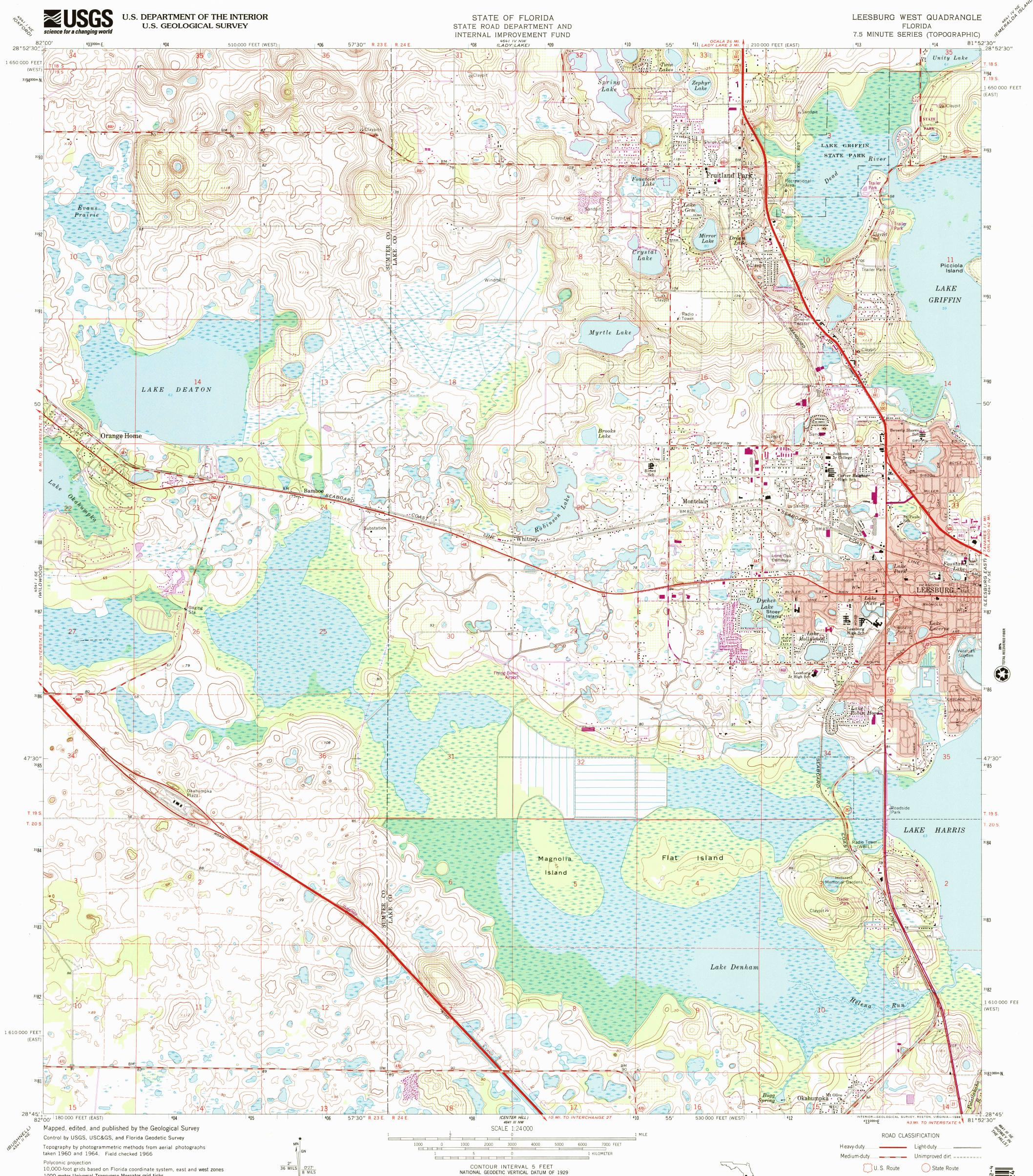
10,000-foot grids based on Florida coordinate system, east and west zones 1000-meter Universal Transverse Mercator grid ticks, zone 17, shown in blue. 1927 North American Datum To place on the predicted North American Datum 1983 move the projection lines 26 meters south and 17 meters west as shown by dashed corner ticks
