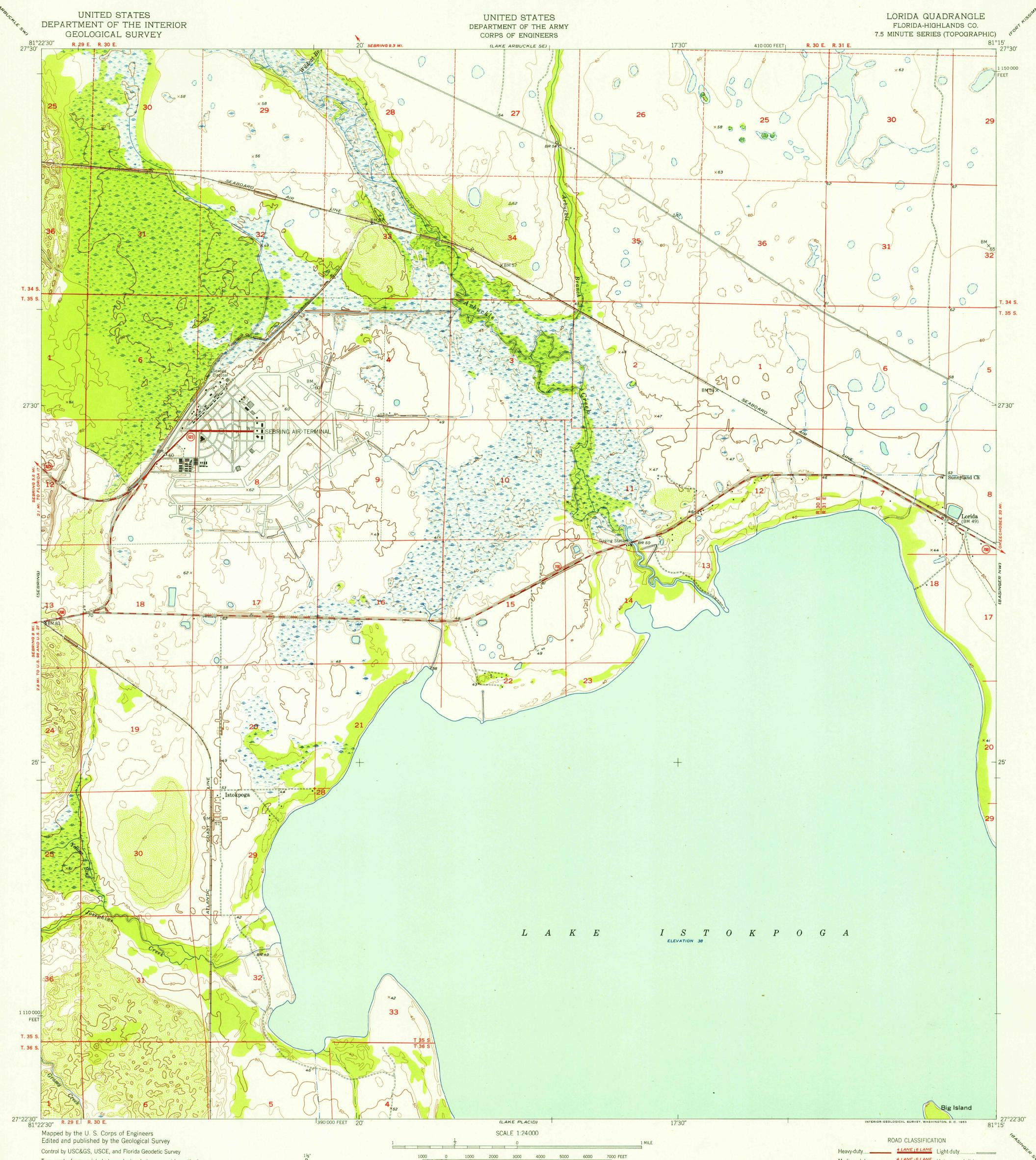
Topography from aerial photographs by photogrammetric methods and by plane-table surveys 1950–1951. Aerial photographs taken 1950 Field check by the Geological Survey 1952
