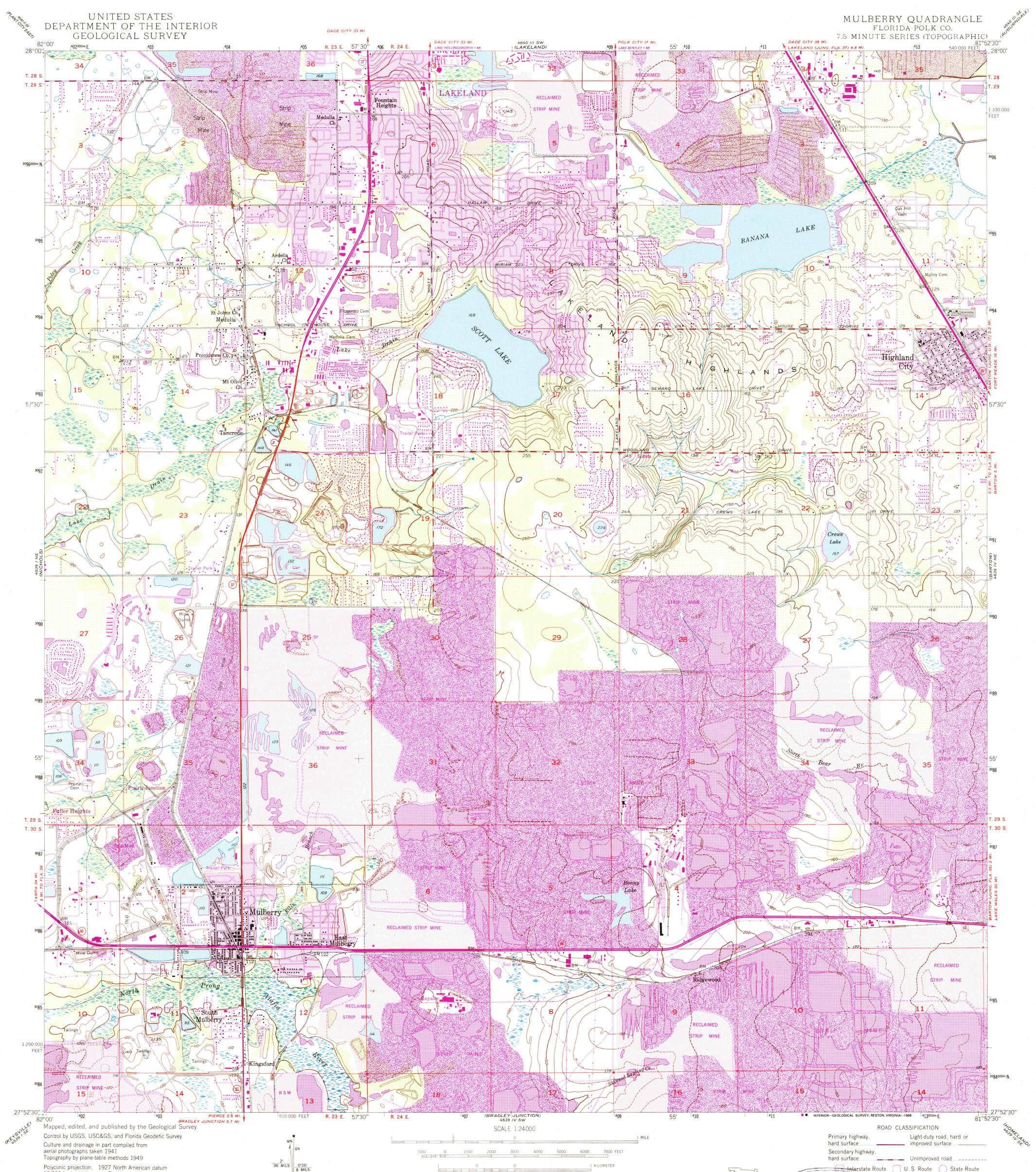
Polyconic projection. 1927 North American datum 10,000-foot grid based on Florida coordinate system, west zone 1000-meter Universal Transverse Mercator grid ticks, zone 17, shown in blue To place on the predicted North American Datum 1983 move the projection lines 29 meters south and 18 meters west as shown by dashed corner ticks Purple tint indicates extension of urban areas
