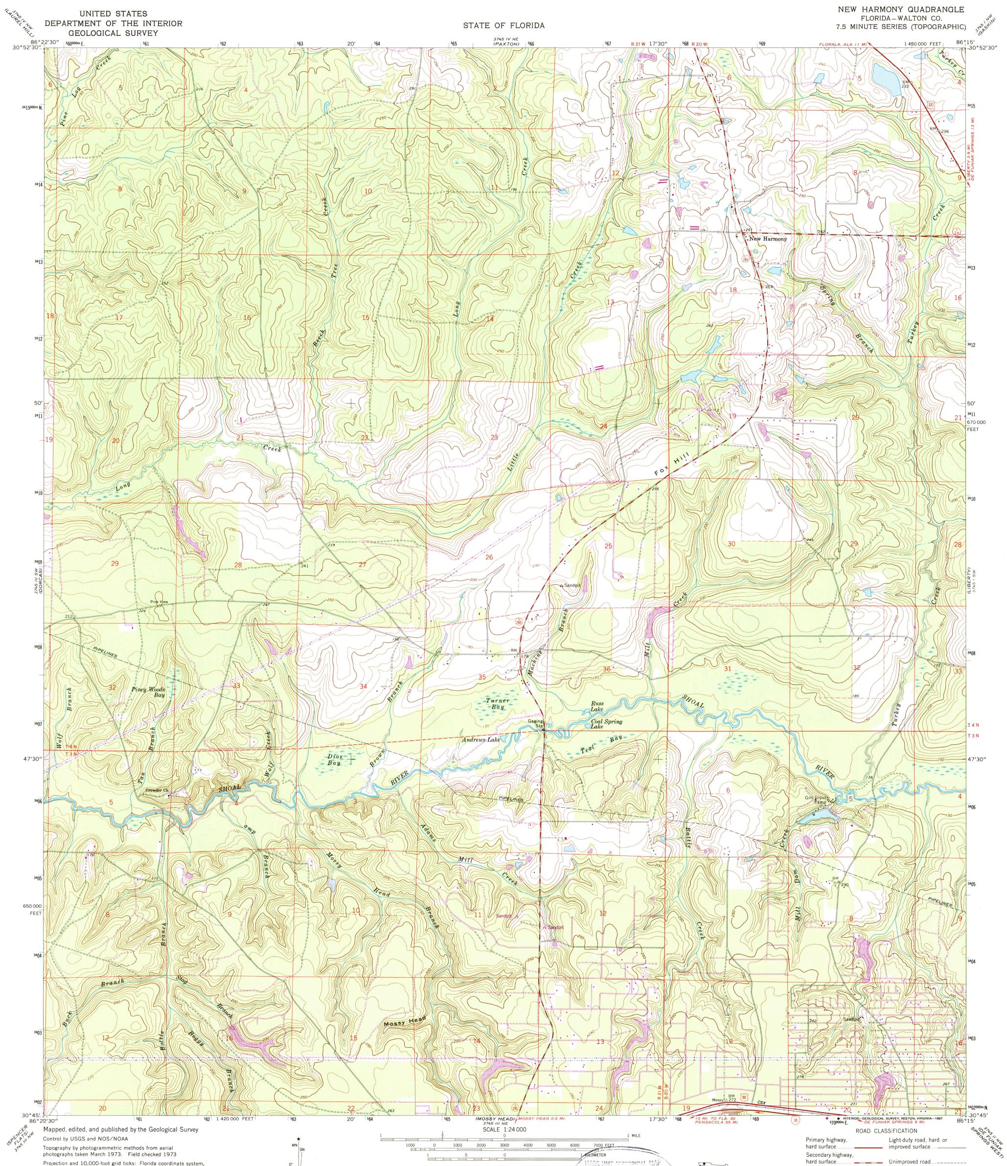
north zone (Lambert conformal conic) 1000-meter Universal Transverse Mercator grid ticks, zone 16, shown in blue. 1927 North American Datum To place on the predicted North American Datum 1983 move the projection lines 16 meters south and 5 meters west as shown by dashed corner ticks
