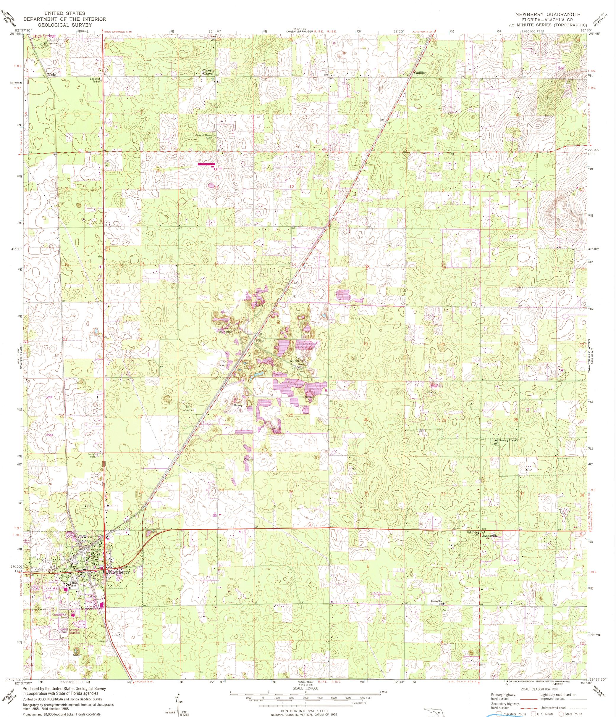
Projection and 10,000-foot grid ticks: Florida coordinate system, north zone (Lambert conformal conic) 1000-meter Universal Transverse Mercator grid ticks, zone 17, shown in blue 1927 North American Datum (NAD 27)
