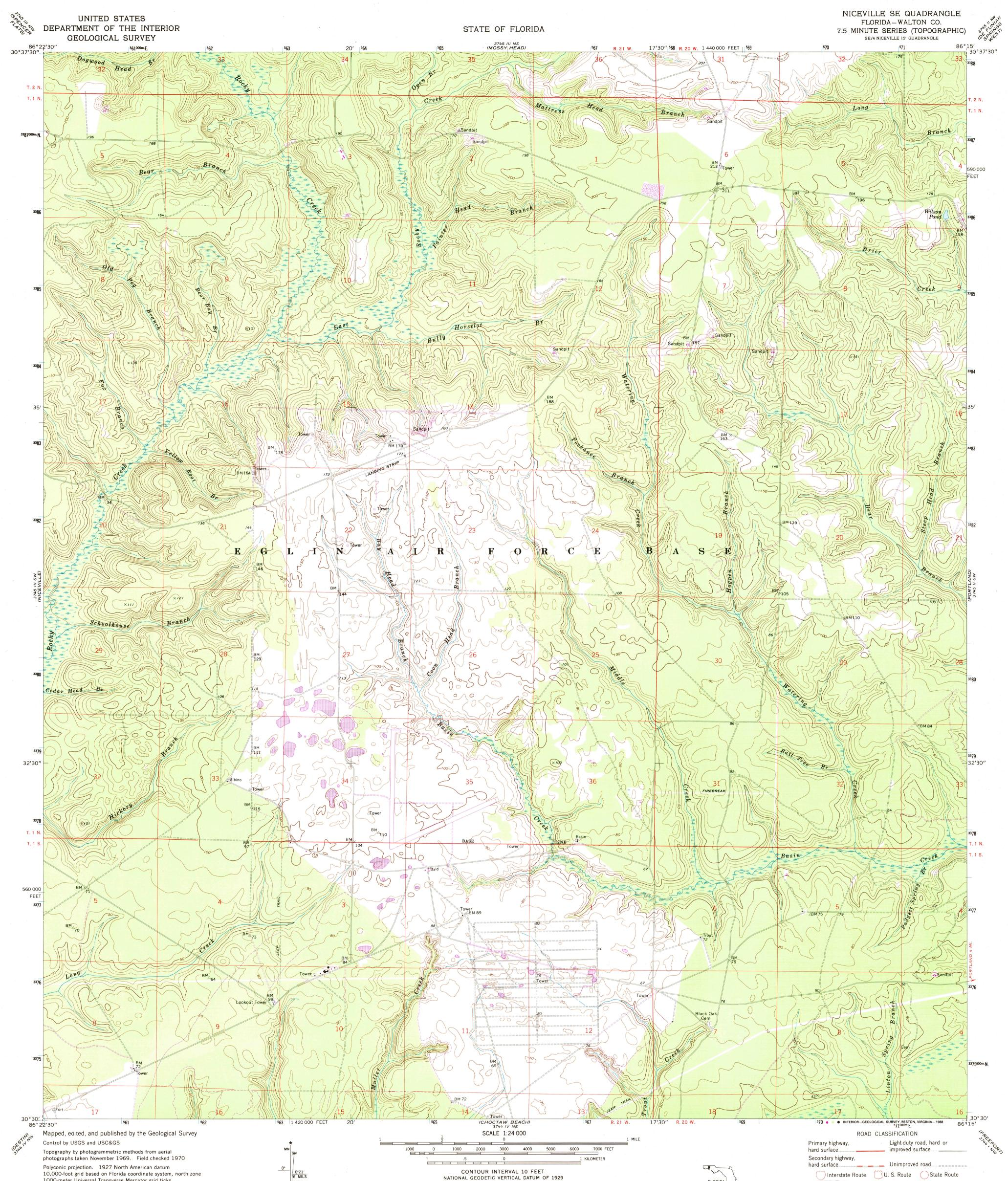
10,000-foot grid based on Florida coordinate system, north zone 1000-meter Universal Transverse Mercator grid ticks, zone 16, shown in blue To place on the predicted North American Datum 1983 move the projection lines 17 meters south and 5 meters west as shown by dashed corner ticks There may be private inholdings within the boundaries of the National or State reservations shown on this map
